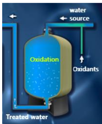
Figure 2.3: Schematic Diagram of Oxidation Process in Wastewater Treatment (EPA, 2015)
