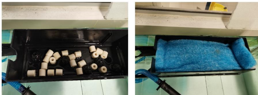
Figure 3.7: Top Filter with Bio-medias and Filter Floss.
