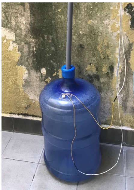
Figure 4.1: Storage Tank used in the Automated RWHS
