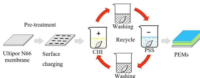
Figure 4.1: Deposition Method for CHI/PSS Layers.
