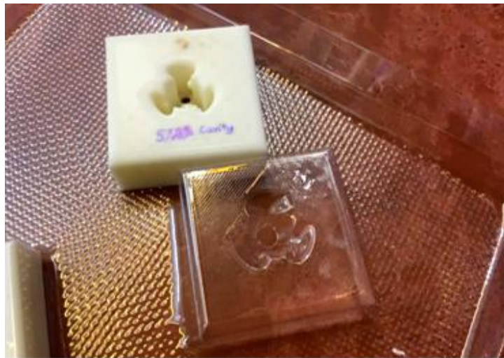
Figure 4.36: Thermoformed Key Tray with 5% of Cavity
