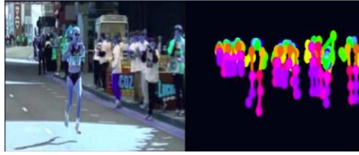
Figure 3.2: The image shown on the left is the original video frame before pose estimation; the image on the right shows pose keypoints of the pedestrians drawn on the black canvas after pose estimation.
