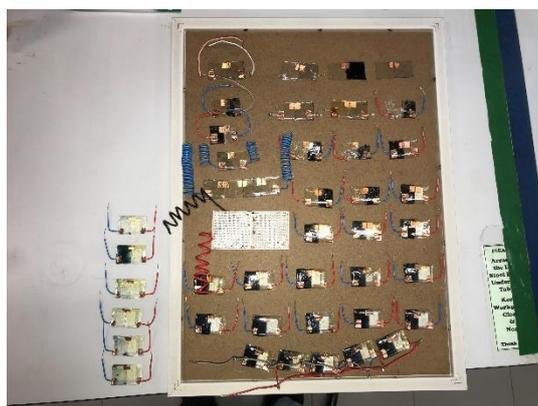
Figure 4.20: Some Samples of Fabricated TEGs.
