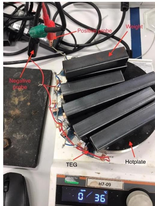
Figure 4.13: Five TEGs Connected in Parallel.
