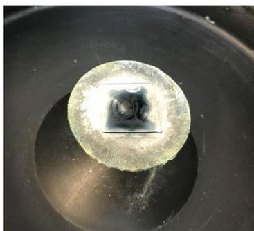
Figure 3.4: 70  $\mu\text{L}$  PEDOT:PSS Solution on Glass Substrate.
