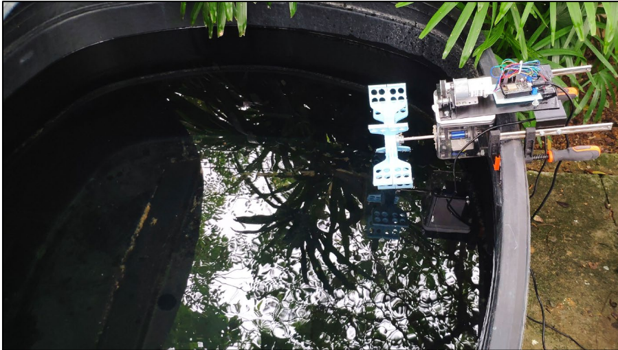
Figure 4.5: Aerator with Impeller 1.
