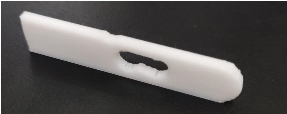
Figure 4.38: Actual 3D printed bracket.
