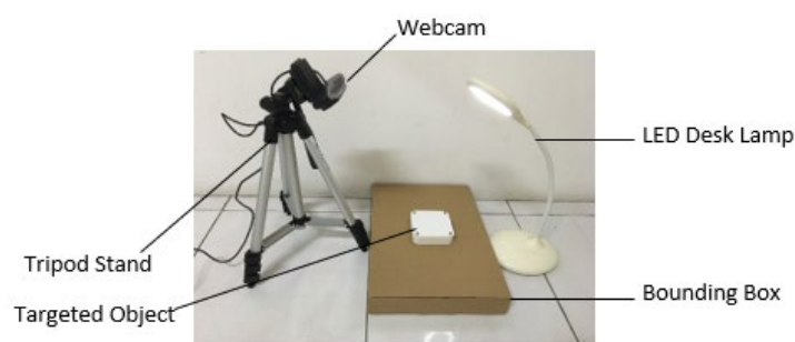
Figure 3.11: Webcam-based Object Detection Setup.
