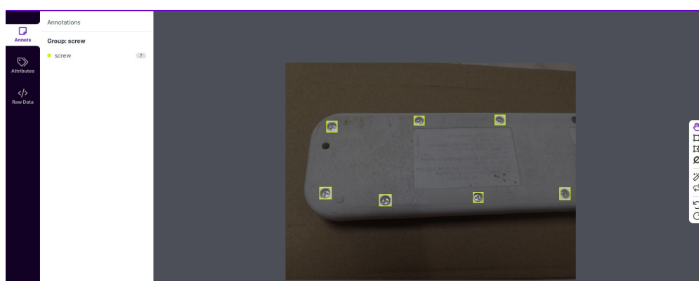
Figure 3.6: Data Annotation in Roboflow Software.
