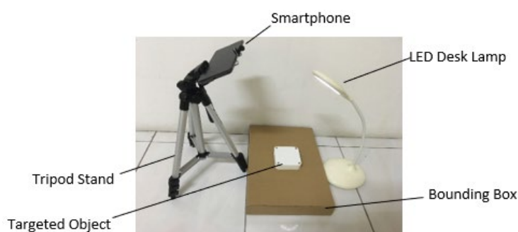
Figure 3.10: Smartphone-based Object Detection Setup.
