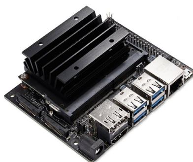
Figure 3.25: Jetson Nano (NVIDIA, 2014)
