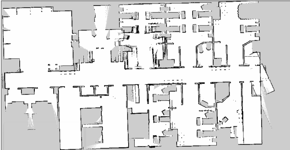
Figure 4.21: Map is Distorted due to Collision.
