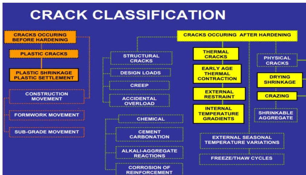
Figure 2.1: Types and Reasons for Cracking (Stanley, 2009)
