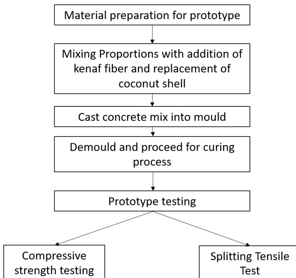
Figure 3.1: Overview of casting work
