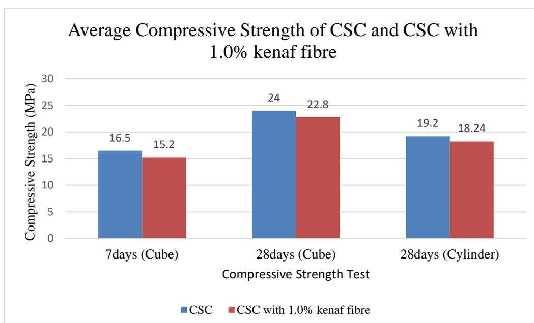
Figure 4.1: Average Compressive Strength of CSC and CSC with 1.0% kenaf fibre
