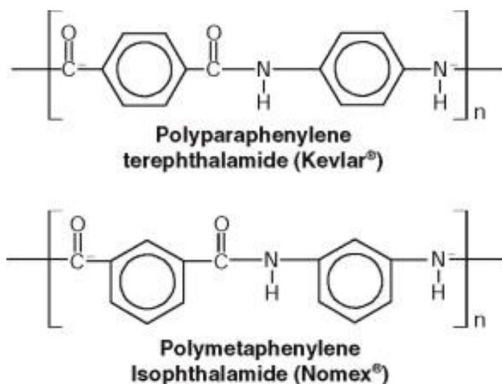
Figure 2.9: Para and Meta Type of Aramid Fibre (Prasad et al., 2014)
