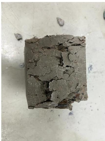
Figure 4.2: Crack Pattern of CSC
