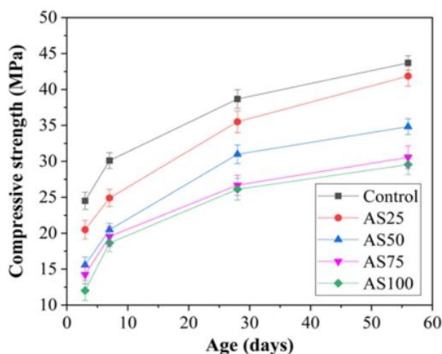
Figure 2.5: Compressive strength of concrete with different apricot shell content (Wu et al., 2019)
