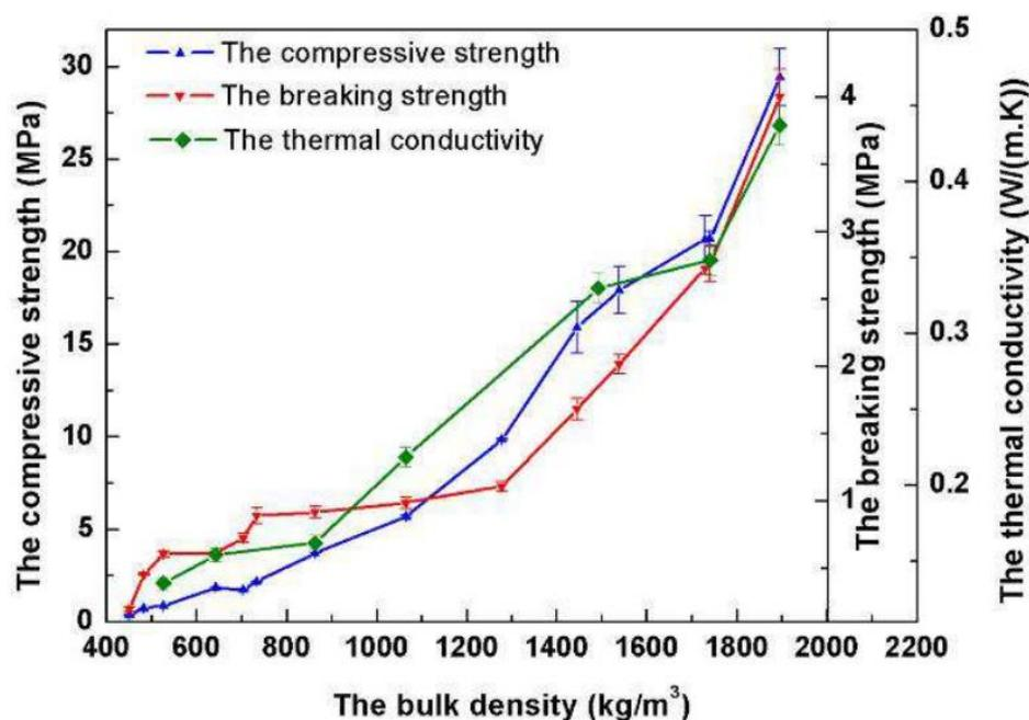
Figure 2.4: The strong performance of lightweight concrete with different proportions of expanded perlite (Ji et al., 2015)
