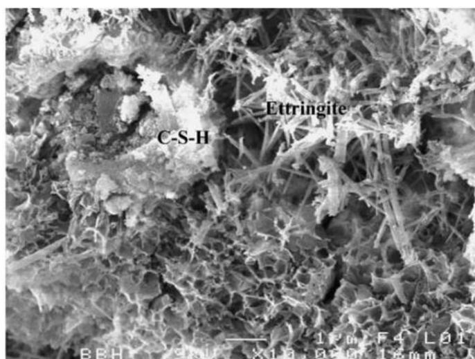
Figure 2.6: Ettringite needles developed on cement matrix's surface (Coatanlem, Jauberthie and Rendell, 2006)
