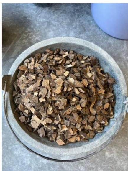
Figure 3.3: Coconut Shell Aggregate
