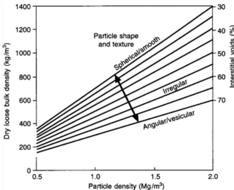
Figure 2.2: Relationship of particle density versus dry loose bulk density determines the characteristic of a particle on the effect of interstitial void on lightweight aggregates (Lclarke, 1993).
