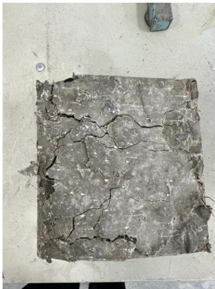
Figure 4.3:Crack Pattern of CSC with 1.0% Kenaf Fibre
