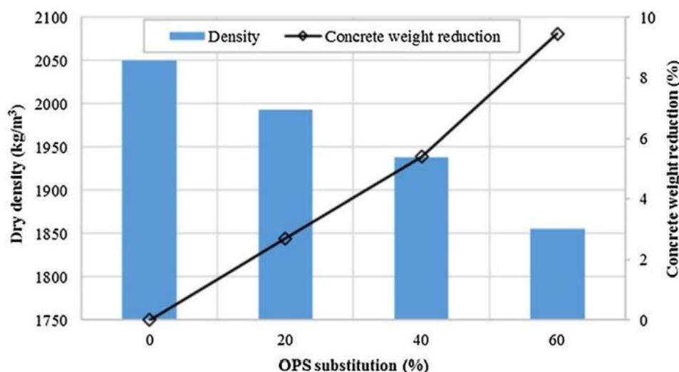
Figure 2.7: Relationship between the proportion of palm shell substitution versus dry density of concrete(Hamada et al., 2020)
