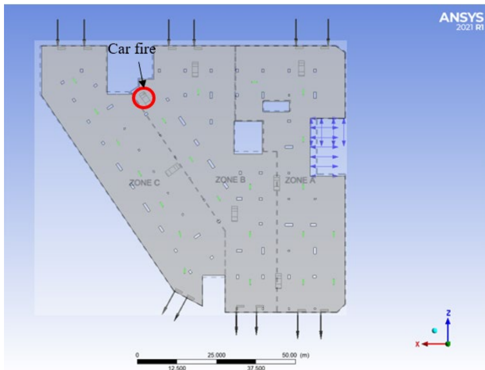
Figure 3.14: Boundary settings of jet fans ventilation system
