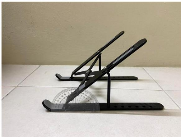
Figure 3.47: Laptop stand with adjustable height for topple angle testing
