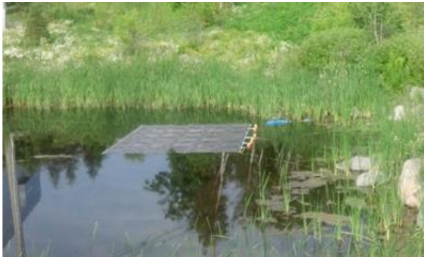
Figure 2.4: Floating PV panel designed by MIRARCO (Trapani and Redón Santafé, 2014)
