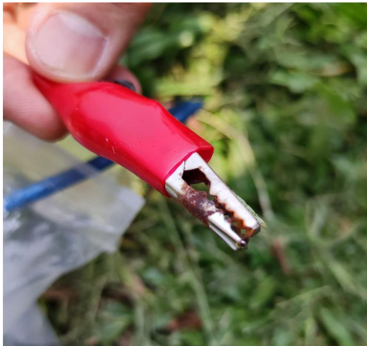
Figure 4.35: Rusted Crocodile Clip on GPV after one week
