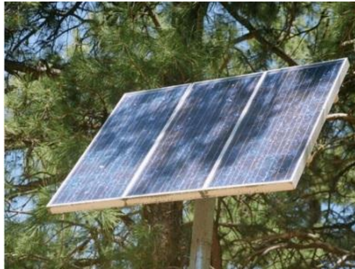
Figure 2.2: Partially shaded PV module (Dwivedi, Yadav and Saket, 2016)
