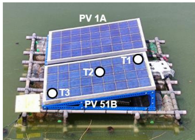
Figure 3.34: Position of temperature sensors on FPV system
