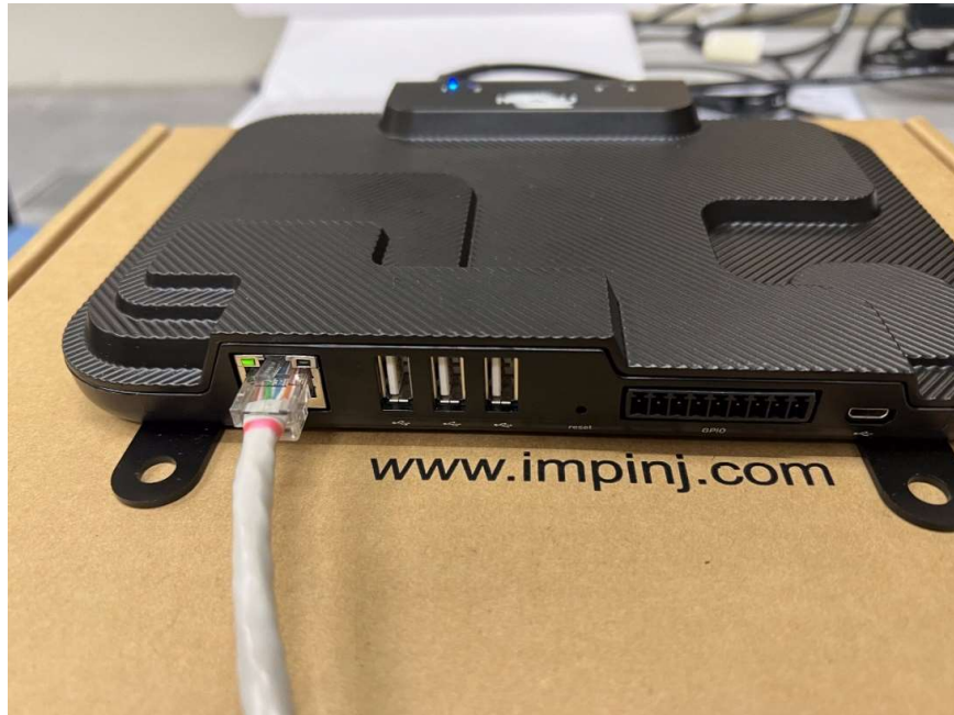
Figure 4.1.2.4 OUT port is connected to the RFID reader.
