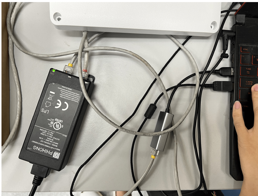
Figure 4.1.2.5 IN port is connected to the laptop via the USB-ethernet converter.
