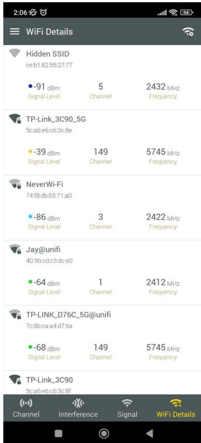
**Figure 2.8 Wi-Fi Details Given by The Wi-Fi Analyzer and Surveyor**
