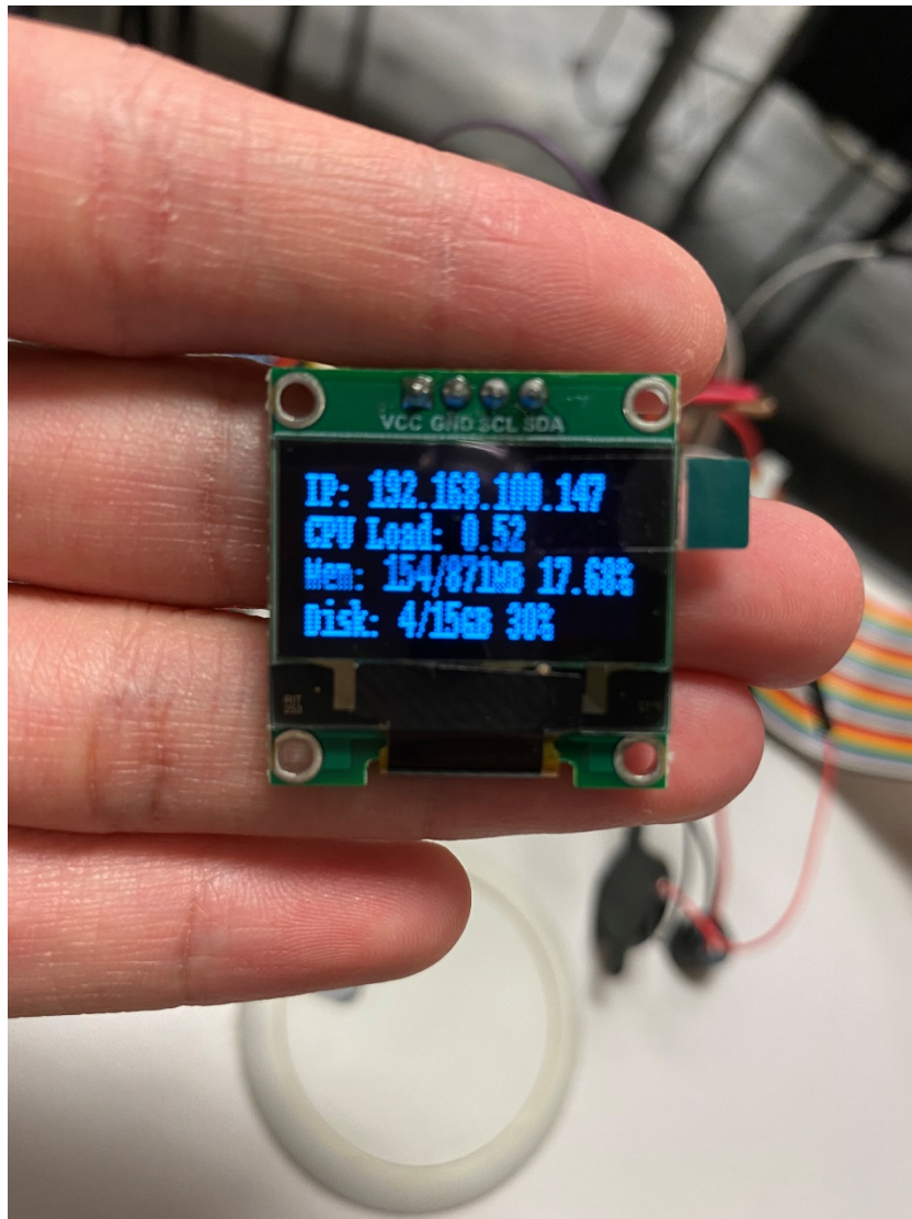
Figure 5.1.11: Sample Output from 0.96-inch OLED Display.
