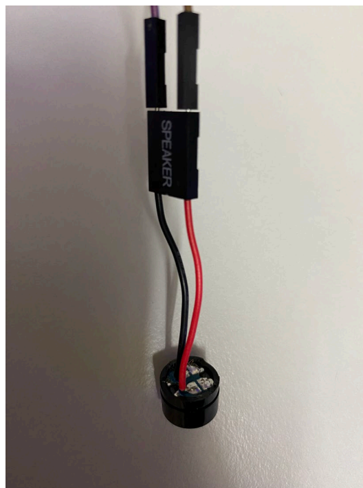
Figure 5.4.8 Buzzer Produce Alert.
