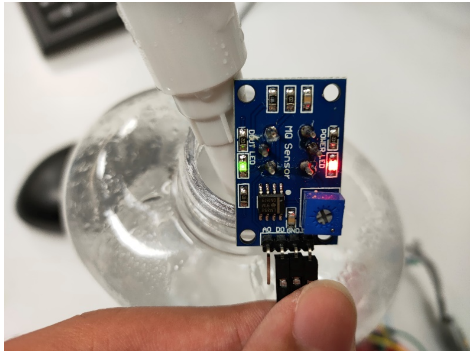
Figure 6.3 MQ135 detected dangerous gas or flammable gas
