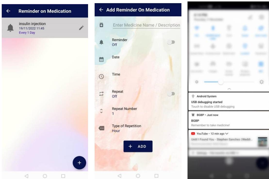
Figure 6.9: RecyclerView for medication record (Left); Add reminder on medication interface with textbox, toggle switch to turn on or off the reminder or repetition (Middle); Push notification received as reminder (Right)
