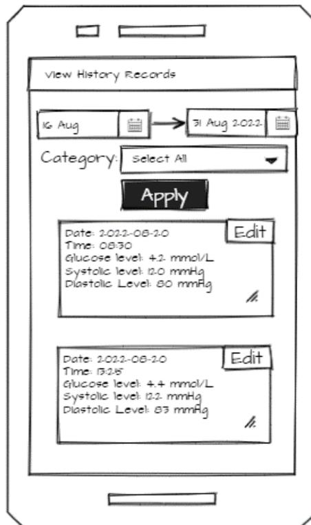
Fig 5.0b: View history records interface where user is able to apply date and category filter and perform modification or deletion on the specific record selected
