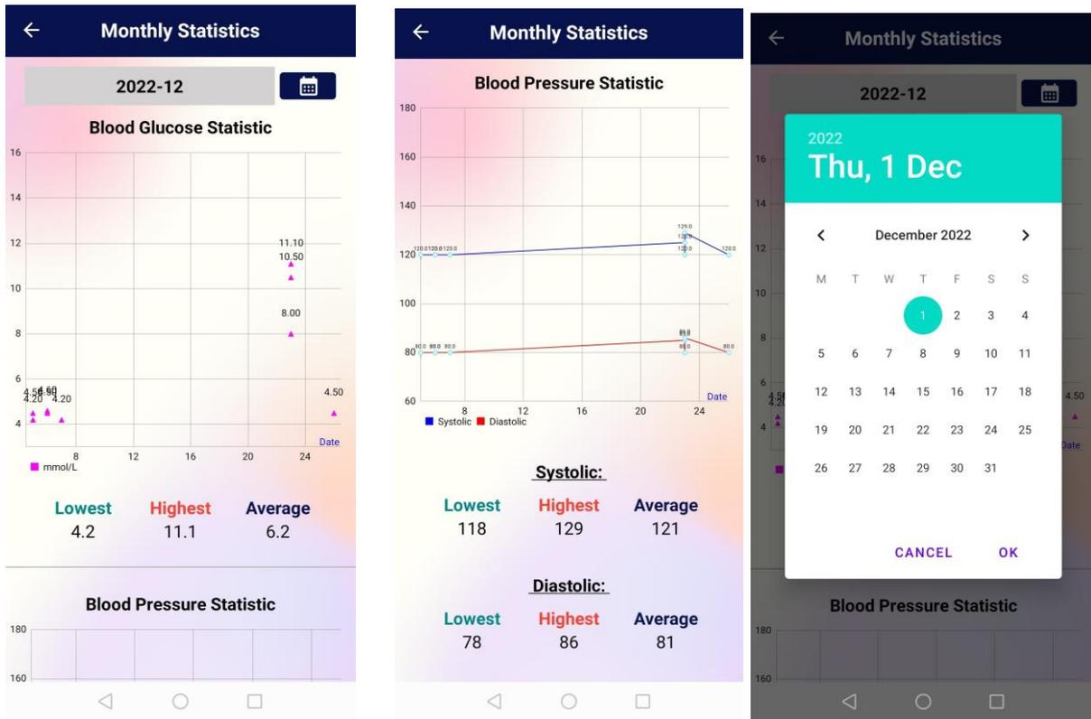
Figure 7.0: Monthly statistics interface (allow user to select the month from DatePickerDialog) and display blood glucose statistic in scatter chart, blood pressure statistic in line chart with the lowest, highest and average data shown for the month
