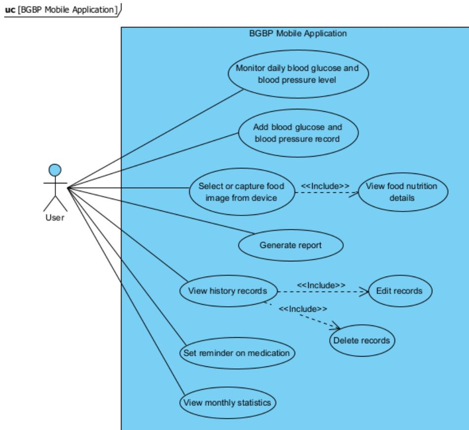
Figure 3.1: Use case diagram for BGBP mobile application by using Visual Paradigm Software
