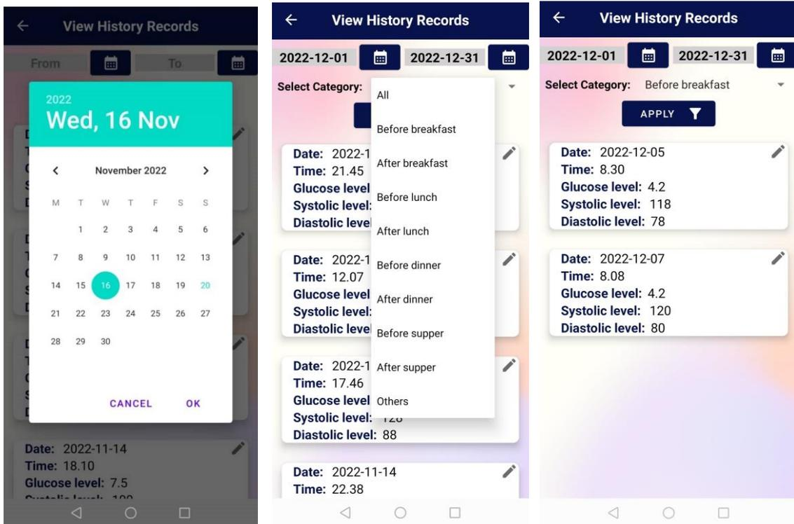
Figure 7.4: History records is also able to apply filter for date range with DatePickerDialog and category filter (for e.g. only showing ‘before breakfast’ records from 01/12/2022 to 31/12/2022 after applied filters)
