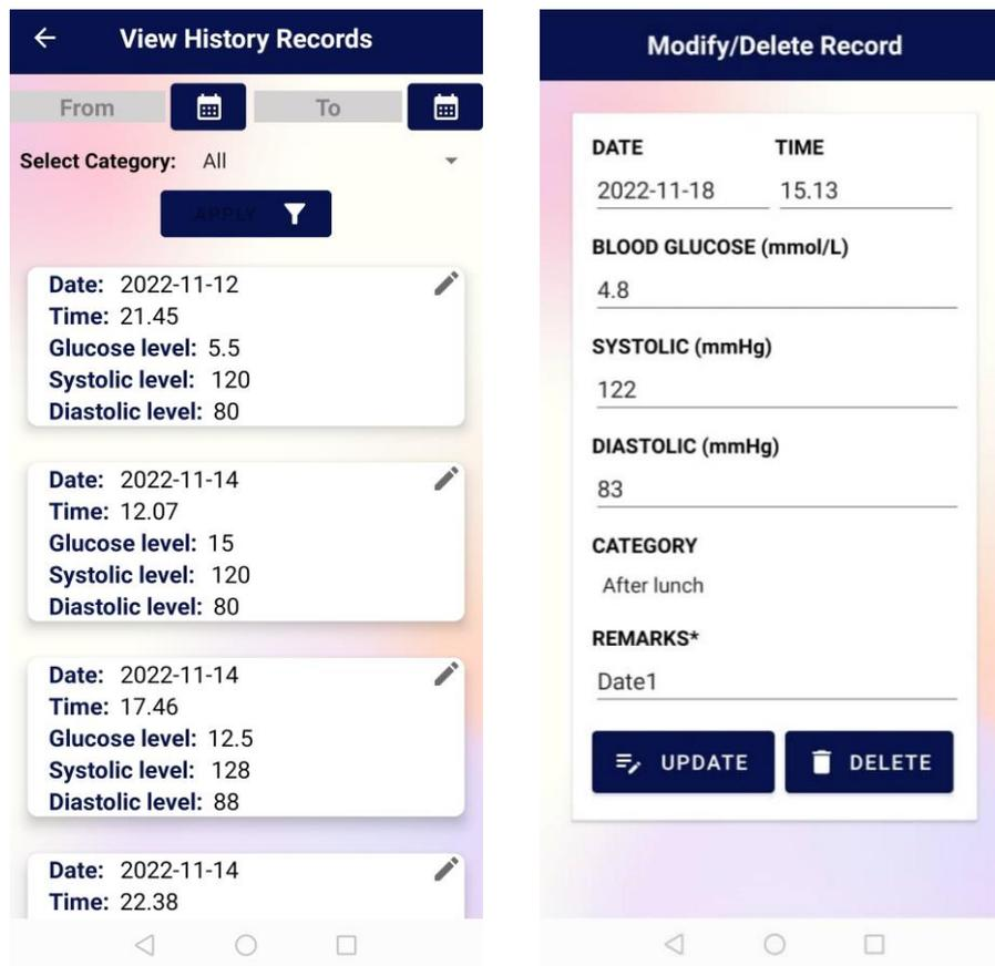
Figure 7.3: History records interface with RecyclerView layout of all records and able to modify or delete the specific record
