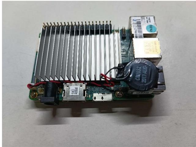
Figure 4.6 Intel UP Board for testing in edge device
