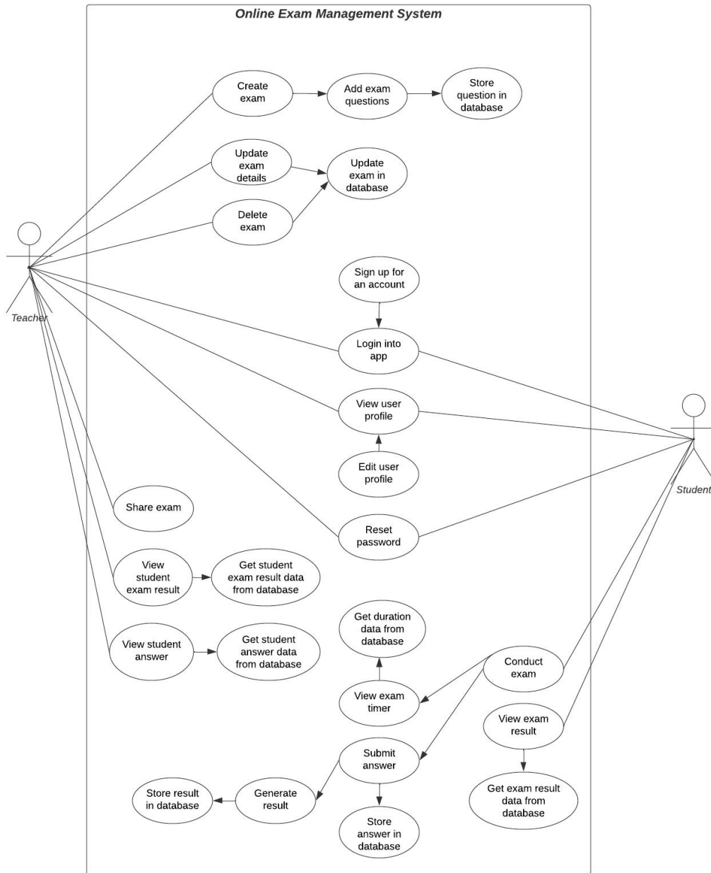
Figure 3.2: Use case diagram of Online Exam Management System
