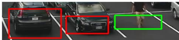
(a) Prediction on some spots 3. The system does get triggered with a human passing through the classification area, which is classified as vacant. The spot 1 and 3 (first two rectangles to the left) are correctly classified as occupied.
