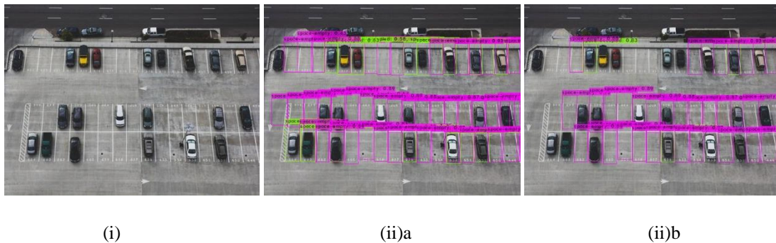
Figure 6.8: Aerial View of Parking Lot (i) test data, (ii) prediction result on the test data with (a) 0.2, (b) 0.7 thresh value
