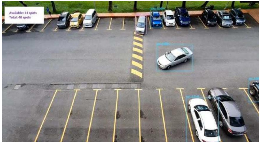
Figure 2.7: Result of YOLOv3 vehicle detection when the vehicle is in-motion [22]
