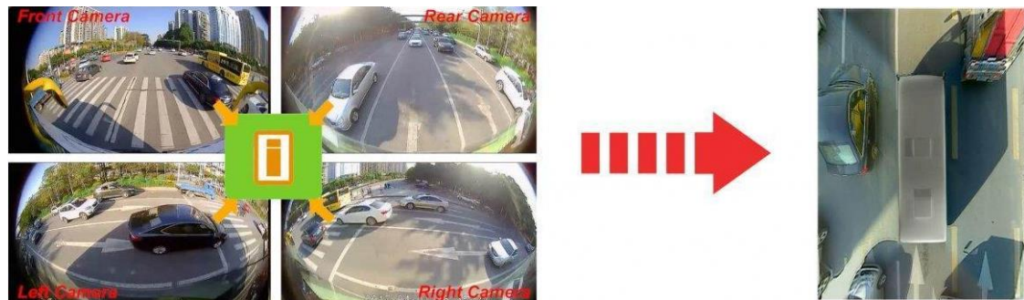
Figure 1.1.2 Diagram above showed how the four-fisheye camera views combined into a top-view image [1].
