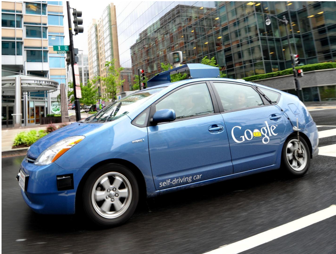
Figure 2.2.2 Diagram above showed the LiDAR component attached on Toyota Prius, and the model's name is called Velodyne HDL-64E LIDAR sensor and cost $75,000 for one LiDAR sensor.
