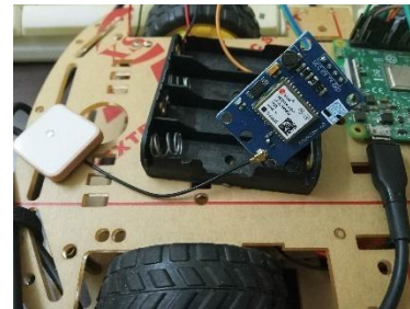
Figure 5.1.4 showed GPS module is connected at the Raspberry Pi 3B+ GPIO pins.
