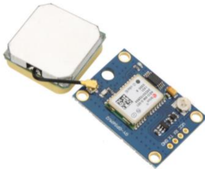
Figure 4.2.1.2 Diagram above showed a sample of GPS Module called “Neo 6M GPS module”.
