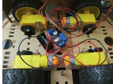
Figure 5.1.2 showed the L298N motor driver is well-connected with 4 DC motors and wheels.
