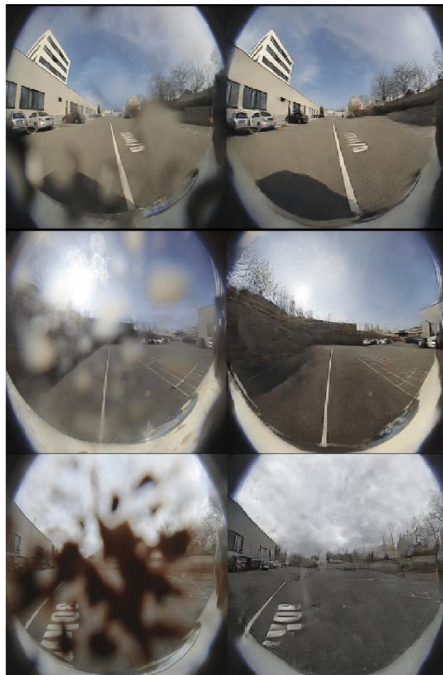
Figure 1.1.3 Diagram showed the unknown sticky liquid blocked the view of camera [2].
