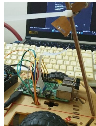
Figure 5.1.4 showed GPS module is connected at the Raspberry Pi 3B+ GPIO pins.
