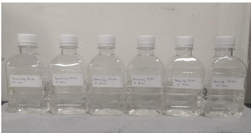
Figure A-2: Effect of Retention Time Using Acid Washed Palm Kernel Shell AC (From sequence of left to right: 20, 40, 60, 80, 100, 120 min).
