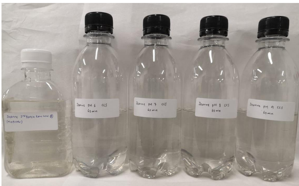
Figure A-6: Effect of Solution pH Using Virgin Coconut Shell AC (From sequence of left to right: raw wastewater, pH 6, pH 7, pH 8, pH 9).
