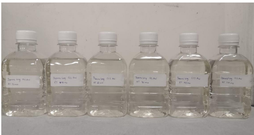
Figure A-4: Effect of Retention Time Using Acid Washed Coconut Shell AC (From sequence of left to right: 20, 40, 60, 80, 100, 120 min).
