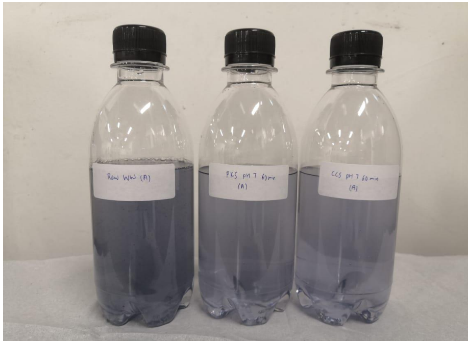
Figure B-1: Final Set of Batch Adsorption Experiment for Sample A Using Virgin Palm Kernel Shell AC and Virgin Coconut Shell AC.
