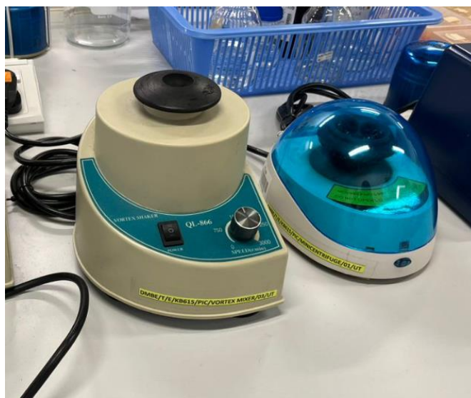
Figure 3.4.3: Vortex Mixer and Minicentrifuge that use to mix the DNA samples and PCR Reagents.
