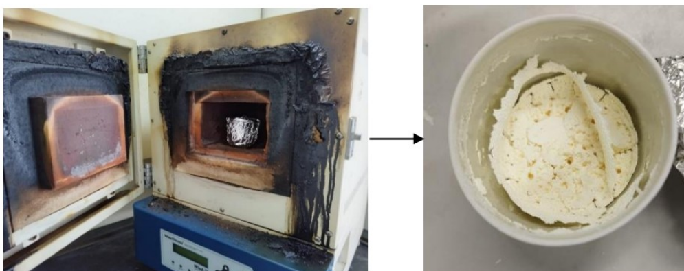
Figure 3.3: Pyrolysis of Urea in Programmable Furnace at 580 °C for 4 h.
