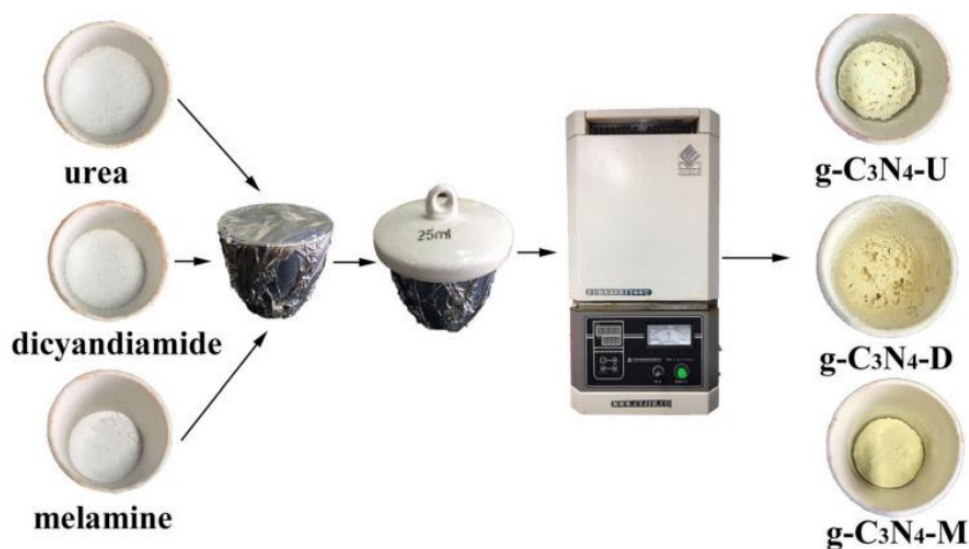
Figure 2.11: General Preparation Process of the Sample of \text{g-C}_3\text{N}_4 using Simple Thermal Polymerization Method (Gao, et al., 2021).
