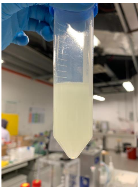
Figure J-13: Sample of Biodiesel Production from Esterification of Oleic Acid and Methanol.
