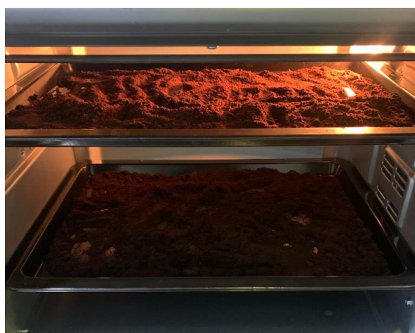
Figure J-2: Dry the Spent Coffee Ground after Washing it with Water.
