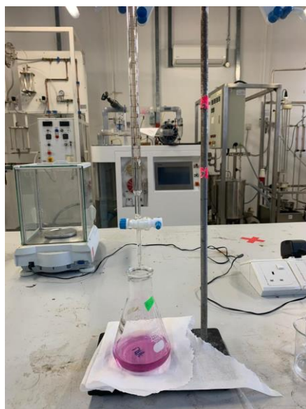
Figure J-11: Apparatus Set-up for Titration to Determine Acid Density of Synthesised Catalyst and Acid Value of Esterification Product.
