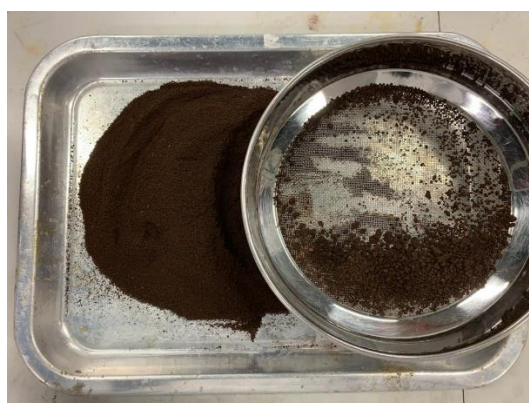
Figure J-3: Sieve the Spent Coffee Ground using Sieve with 600 \mu\text{m} Mesh Size.
