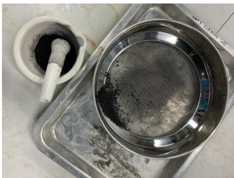
Figure J-8: Further Grinding of Activated Carbon using Sieve with 300 µm Mesh Size.
