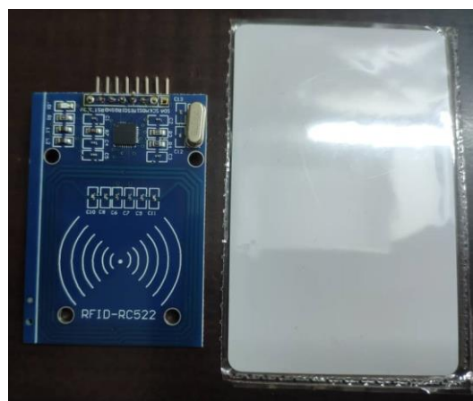
Figure 3.10: RFID Scanner with Model of RC522 at Left and Mifare Card at Right
