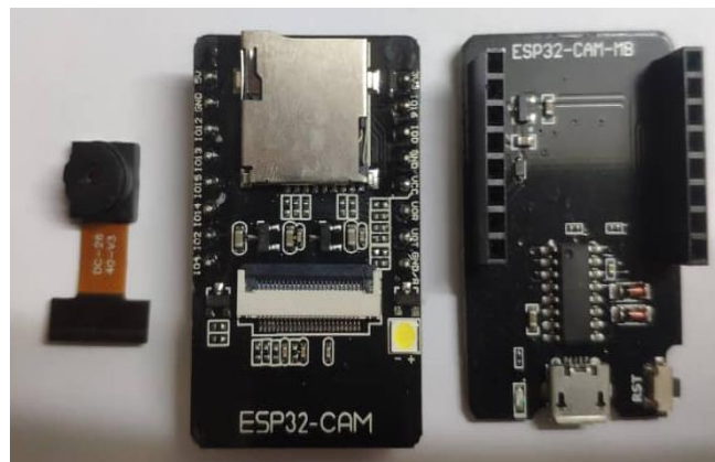
Figure 3.21: Main Parts of Esp32 Cam Module OV2640 Camera at Left, Development Board at Middle, and Programme Unit at Right
