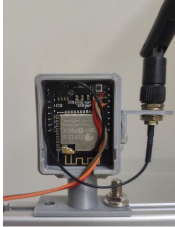
Figure 4.8: Development Board of Esp32 Cam is Solder with Three Wire and Connect to External Antenna
