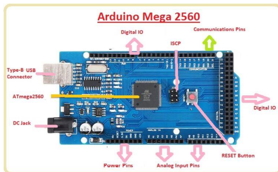
Figure 3.23: Pinout of Arduino Mega 2560 (The Engineering Knowledge, 2023)
