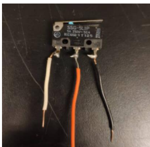
Figure 3.15: Limit Switch with Common Terminal at Left, Normally Open Terminal at Middle and Normally Close Terminal at Right
