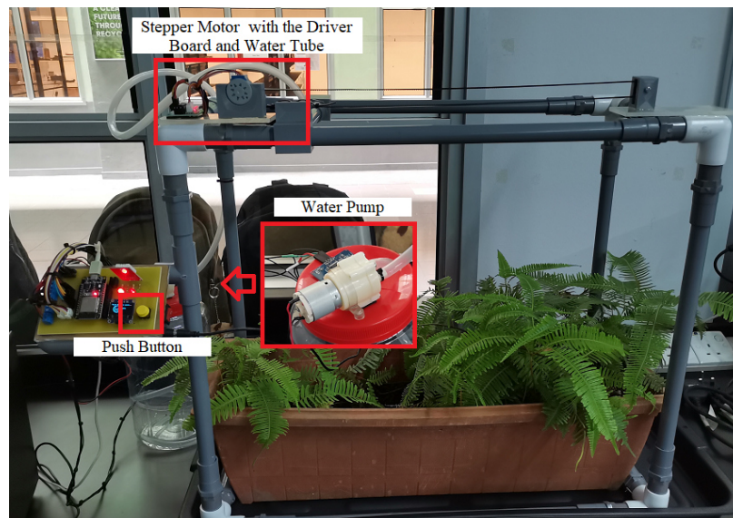
Figure 4.7: Hardware of the Irrigation System
