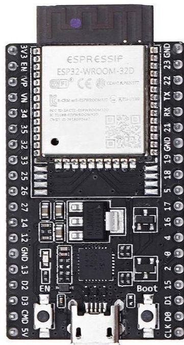
Figure 3.2: ESP32-WROOM-32D Board (Hallroad,2022).
