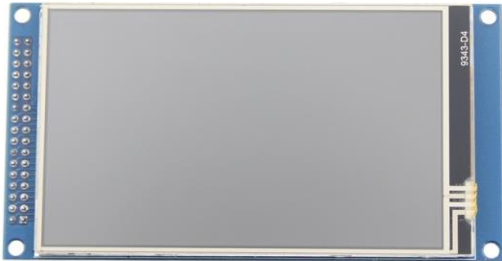
Figure 2.3: OTM8009A Module TFT Screen (LCwiki,2019).
