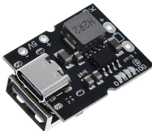
Figure 3.5: Type-C USB 5V 2A Step-up Boost Converter with USB Charger (ShharviElectronic,2022).
