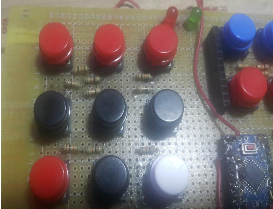
Figure 1.3: The Front View of Stream Deck (NL1_CS, 2019).
