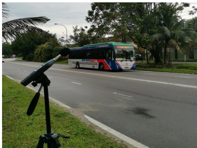
Figure 3.3: Setting Up of Sound Level Meter for Traffic Noise Measurement.
