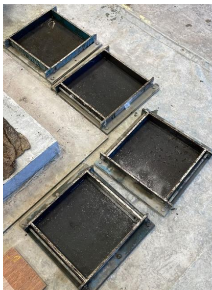
Figure 3.8: Slab Mould Applied with A Layer of Oil.
