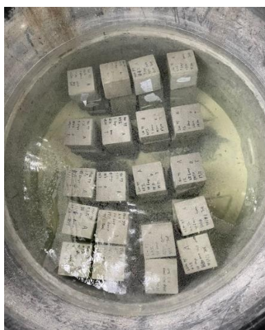
Figure 3.12: Foamed Concrete Samples Being Cured in Water Tank.
