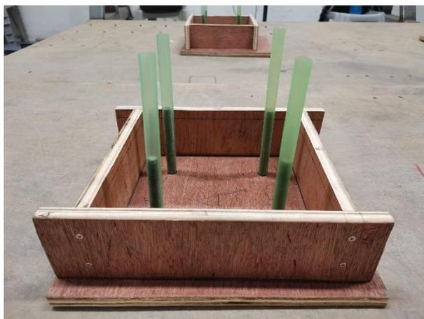
Figure 3.16: Footing Formwork with Bolts Installed on Shaking Table.
