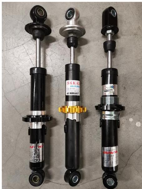
Figure 3.36: APIDO, SKK and ESPADA Dampers (from left to right).
