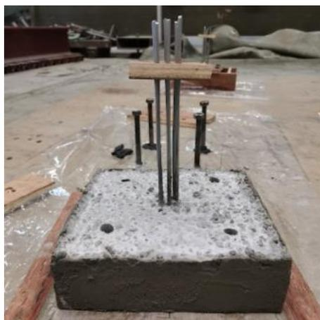
Figure 3.23: Footing Cast.
