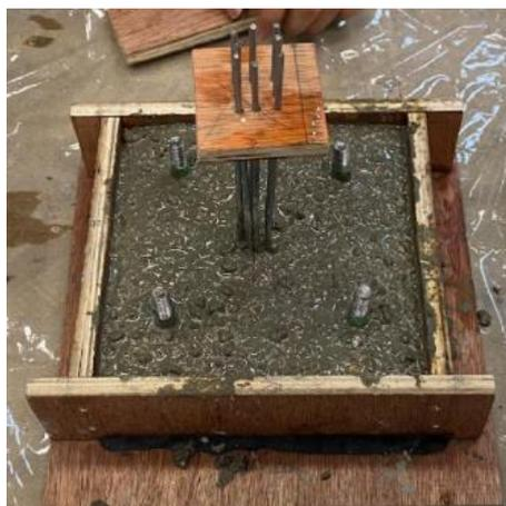
Figure 3.22: Concrete Casting for Footing.
