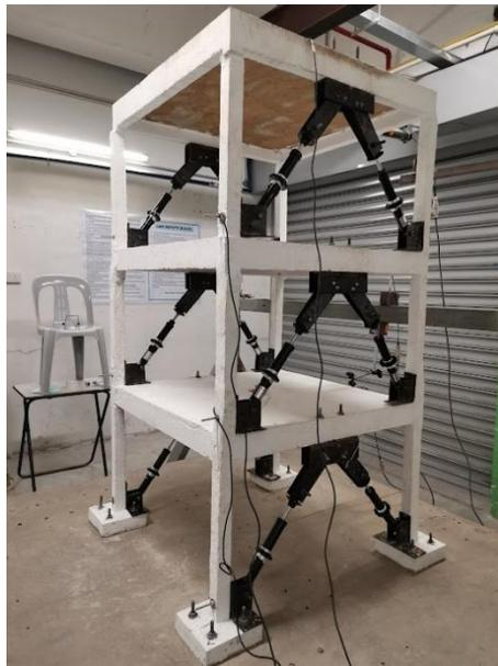
Figure 3.40: Structure with APIDO Dampers Installed on Shaking Table.
