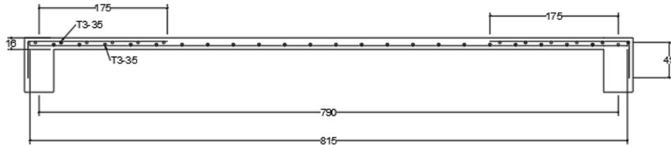
Figure 3.6: Slab Reinforcement Details.
