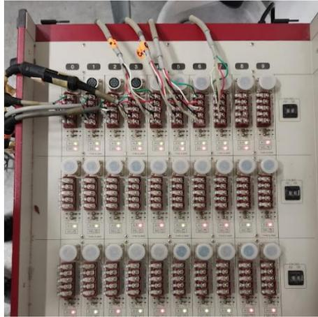
Figure 3.33: Date Logger Connected with the Test Sensors.
