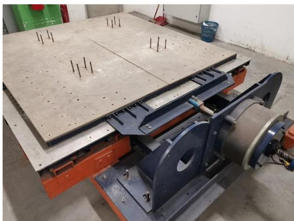
Figure 3.30: Shaking Table in the Advanced Geotechnical Laboratory.
