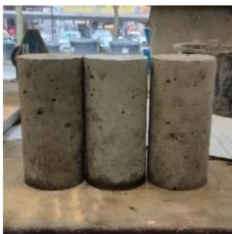
Figure 3.13: Hardened Cylinder Concrete Specimens.
