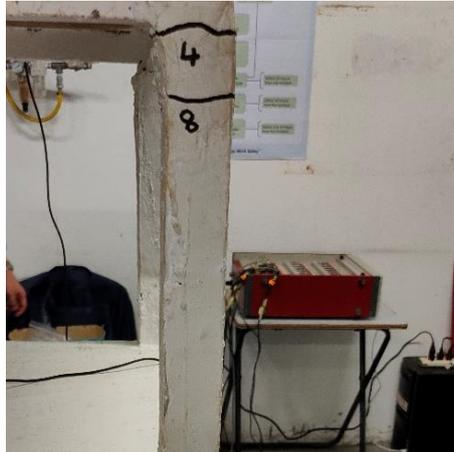
Figure 4.6: Concrete Cracks on the Second Floor Column of Bare Frame Structure.
