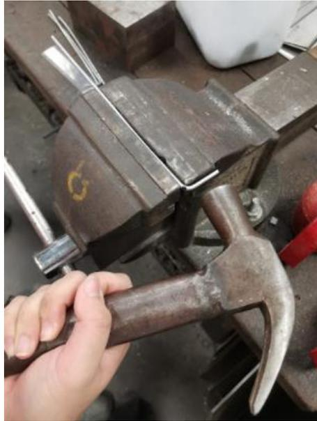
Figure 3.18: Bar Bending in the Mechanical and Timber Workshop.
