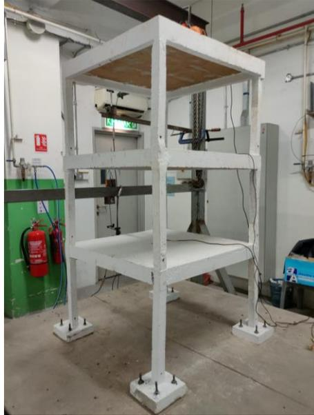
Figure 3.35: Bare Frame Structure Installed on Shaking Table.
