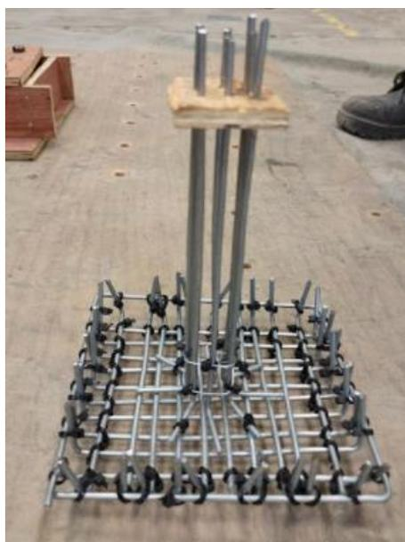
Figure 3.19: Footing Reinforcement with Column Starter Bar.
