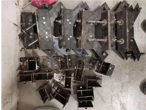
Figure 3.37: Damper Connectors Fabricated for Whole Structure.
