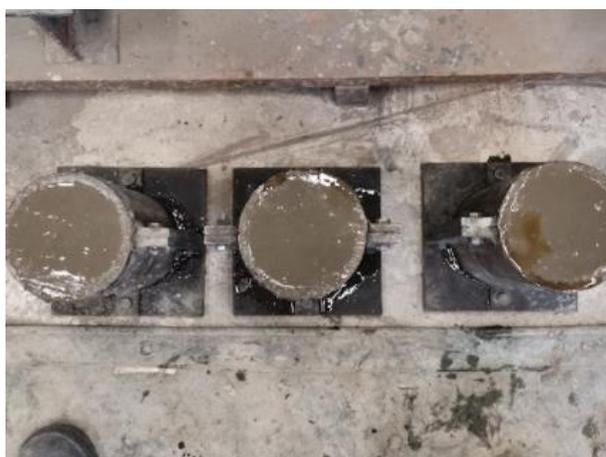
Figure 3.12: Fresh Cylinder Concrete Specimens.
