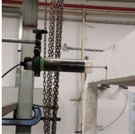
Figure 3.31: 50 mm LVDT Installed on the Third Floor of the Model.
