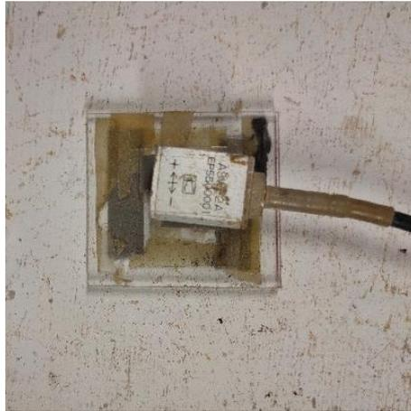
Figure 3.32: Accelerometer Installed on the Third Floor of the Model.
