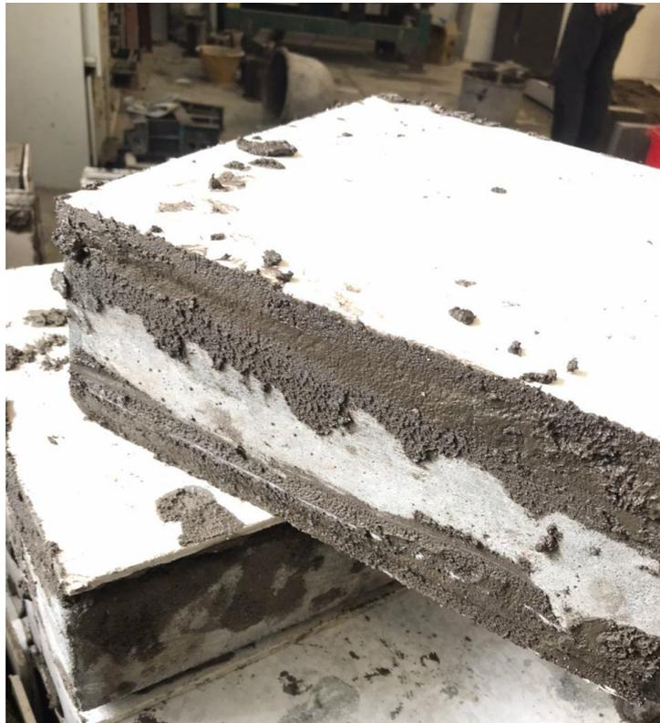
Figure 3.27: Bonding Layer between Magnesium Oxide Board and Concrete.
