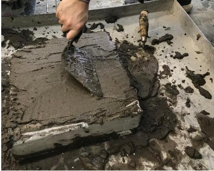
Figure 3.26: Adhesive Applied on Concrete.
