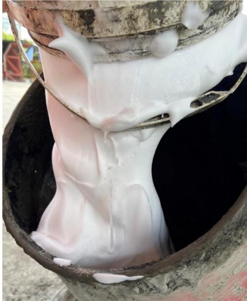
Figure 3.11: Foam Added into Mixture.
