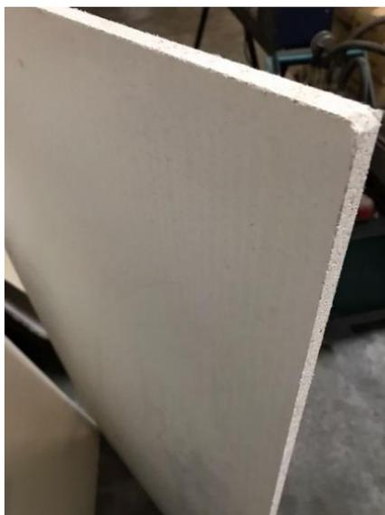
Figure 3.16: Magnesium Oxide Board.
