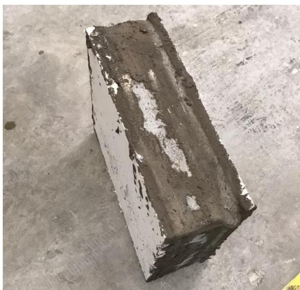
Figure 3.28: Rubberized Lightweight Foamed Concrete Sandwiched Wall Panel.
