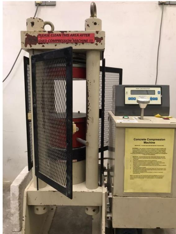
Figure 3.33: Concrete Compression Test Apparatus.
