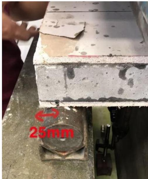
Figure 3.30: 25 mm from Each End of the Specimen at the Centre of the Roller.
