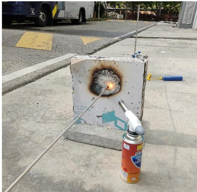
Figure 3.37: Setup of Flame Exposure Test.
