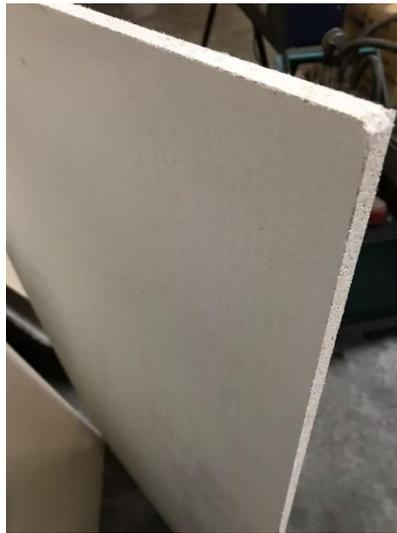
Figure 3.6: Magnesium Oxide Board.
