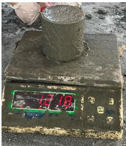
Figure 3.15: Measure the Density of Fresh Mix on Weighing Scale.
