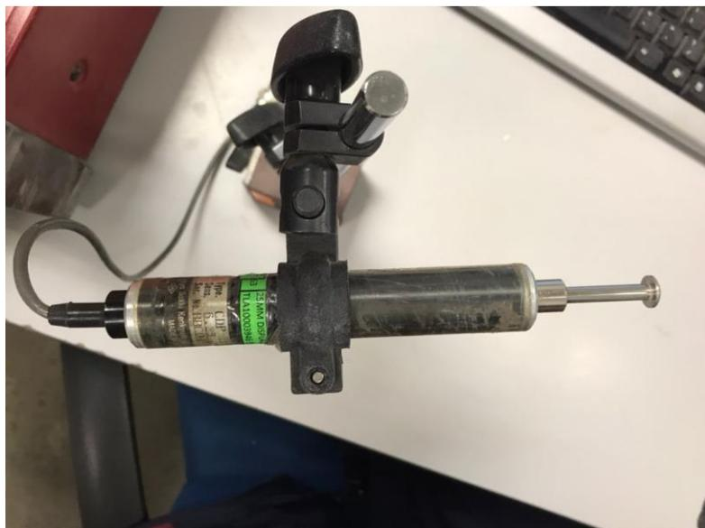
Figure 3.31: Linear Variable Differential Transducer (LVDT).
