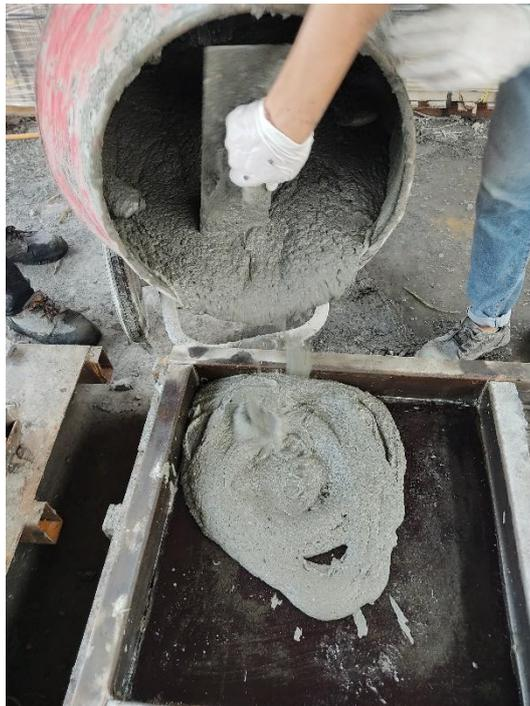
Figure 3.20: Pouring Concrete Mixture to Mould.
