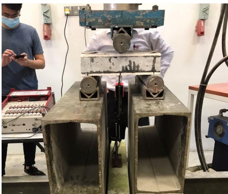
Figure 3.29: Flexural Strength Set Up.
