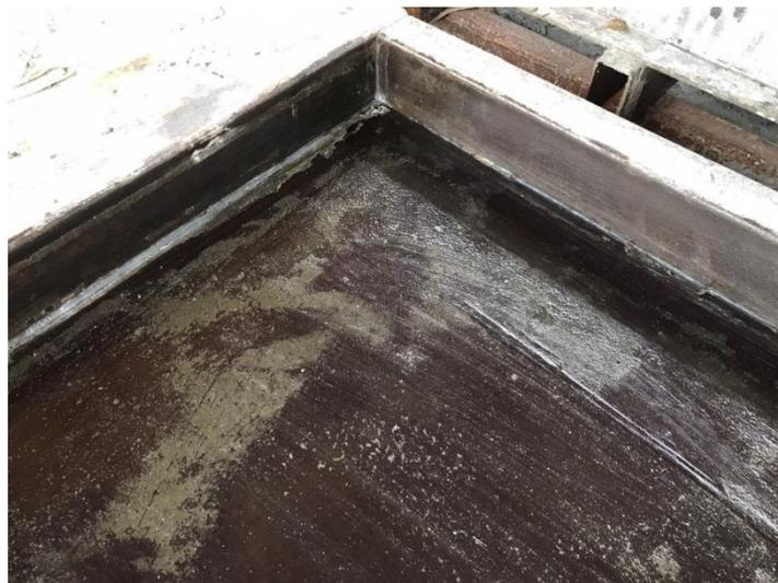
Figure 3.19: Oiled Steel Mould.
