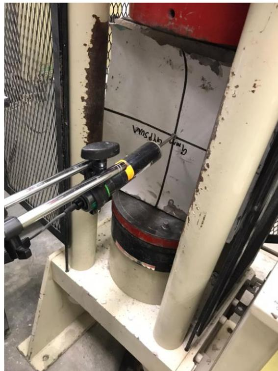
Figure 3.34: Setup of Linear Variable Differential Transducer (LVDT).
