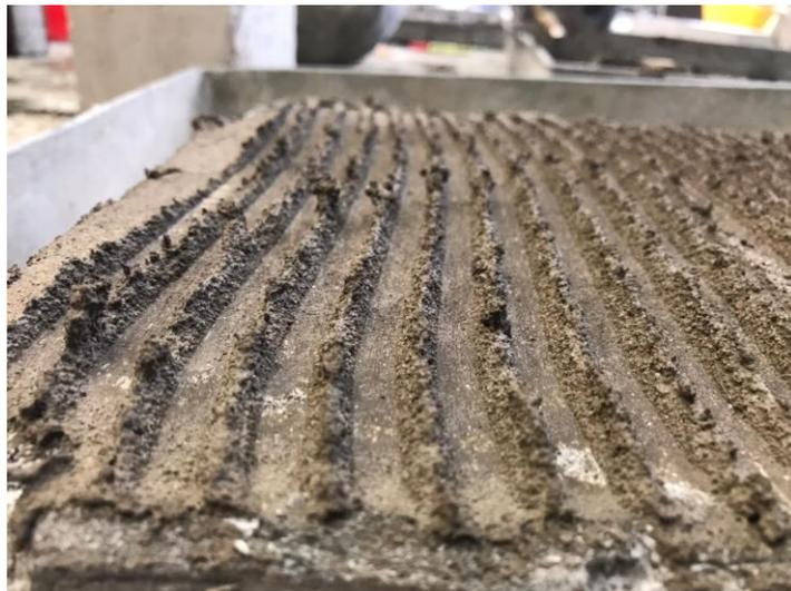
Figure 3.25: Coating on Concrete (Side View).
