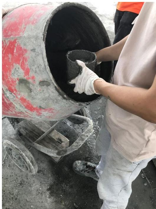
Figure 3.14: Pour Fresh Mix into The Measurement Container.
