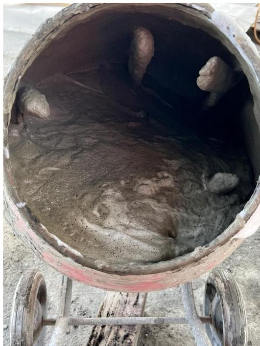
Figure 3.12: Non-Thorough Mix of Foam and Concrete.
