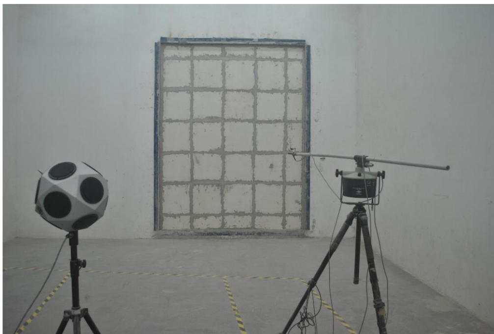
Figure 4.2: Test Setup for Testing the Sandwiched Wall Panel in the Receiving Room.
