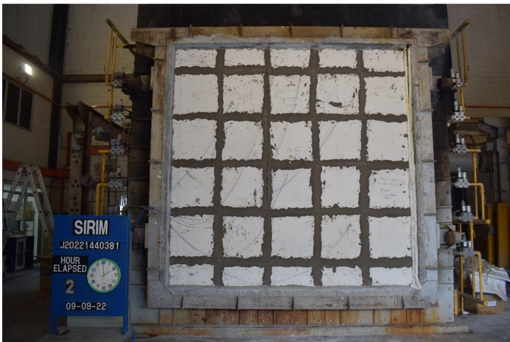
Figure 4.7: The Unexposed Face of the Sandwiched Wall Panel After the Test.
