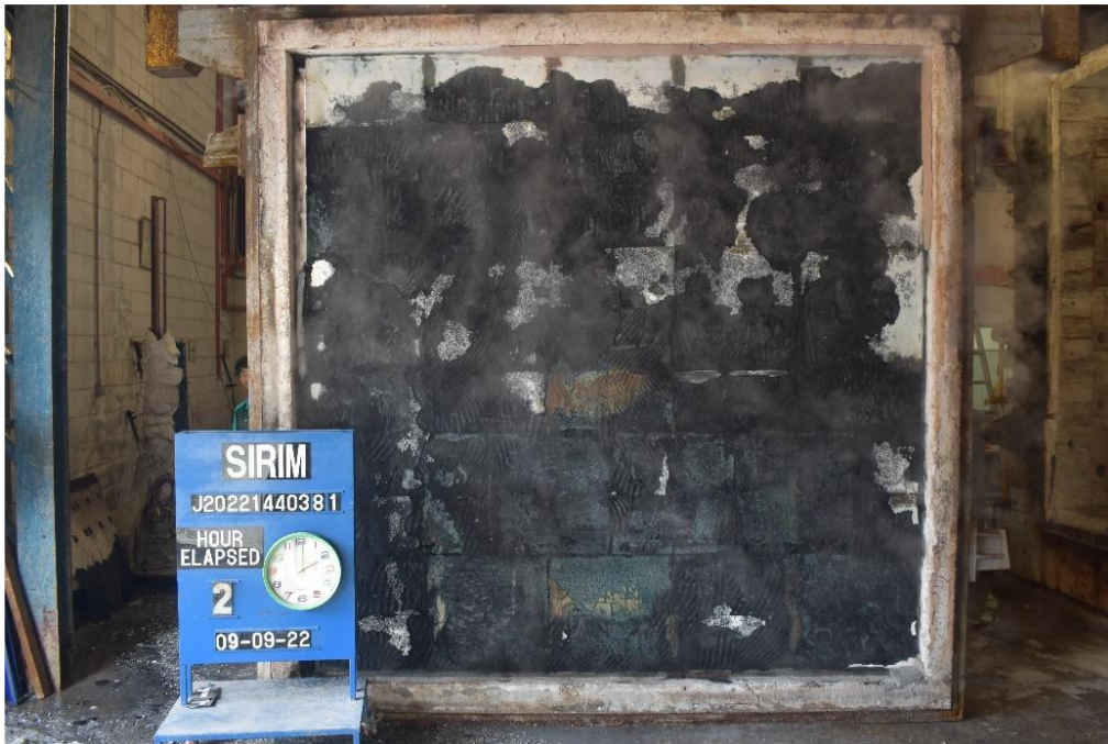
Figure 4.16: The Exposed Face of the Specimen after the Hose Stream Test.
