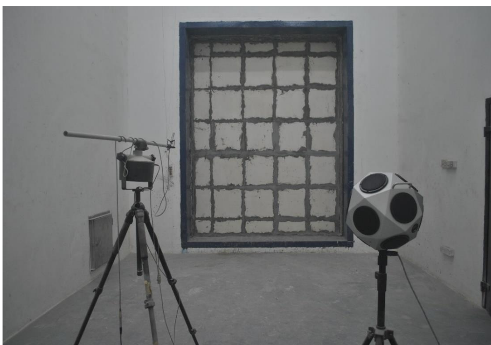
Figure 4.1: Test Setup for Testing of Sandwiched Wall Panel in the Source Room.
