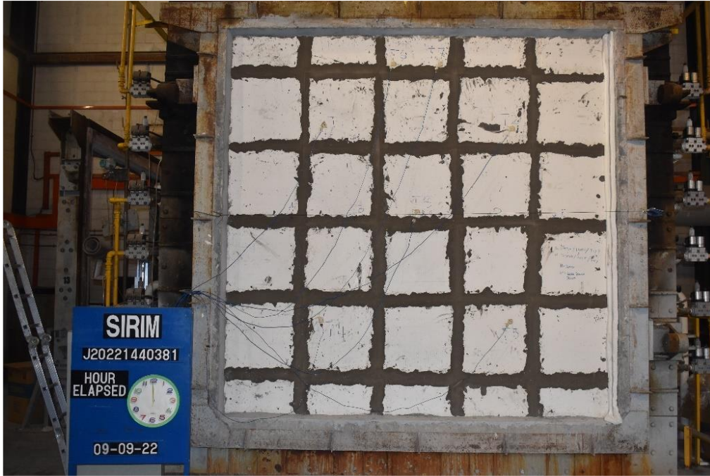
Figure 4.6: The Unexposed Face of the Sandwiched Wall Panel Before the Test.
