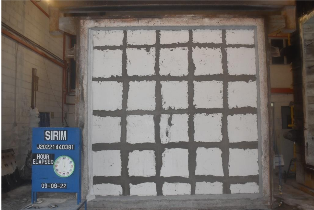
Figure 4.4: The Exposed Face of the Sandwiched Wall Panel Before the Test.
