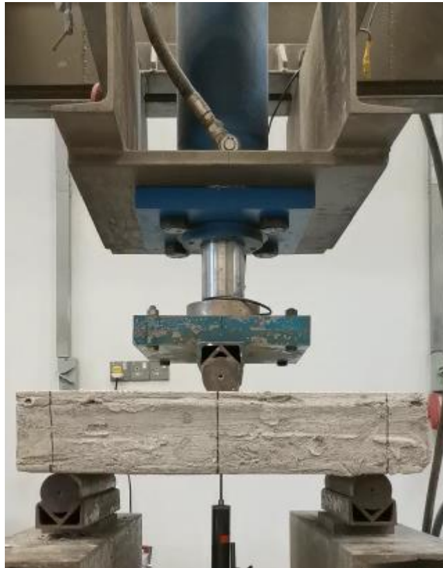
Figure 4.17: Actual Set-up of Flexural Strength Test.
