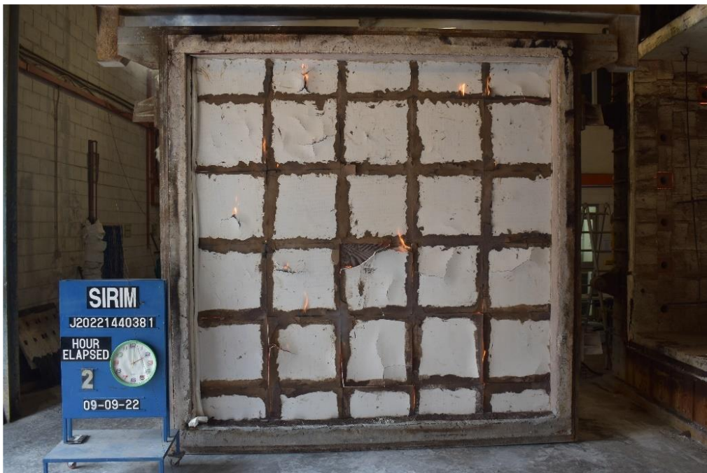
Figure 4.5: The Exposed Face of the Sandwiched Wall Panel After the Test.
