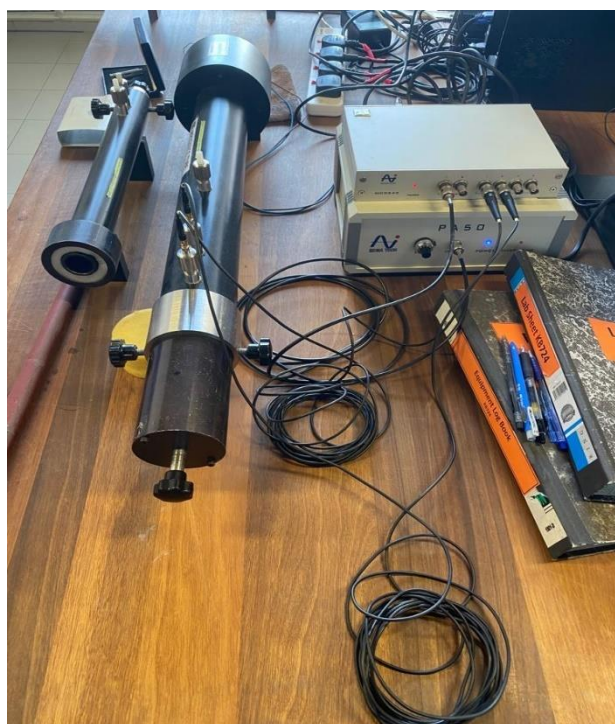
Figure 3.13: Set up of apparatus for Impedance Tube Test.
