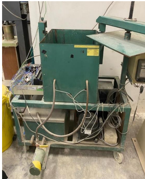
Figure 3.12: Machinery Used for a Thermal Conductivity Test.
