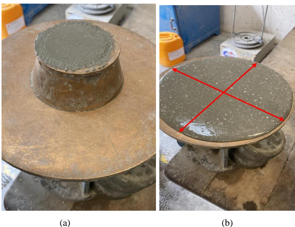
Figure 3.10: Flow Table Test (a) Cone filled with Cement Slurry, (b) Spread of Cement Slurry.
