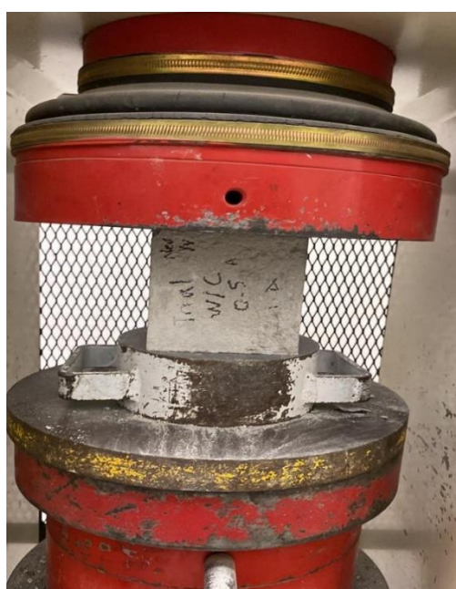
Figure 3.11: Compressive Strength Test.
