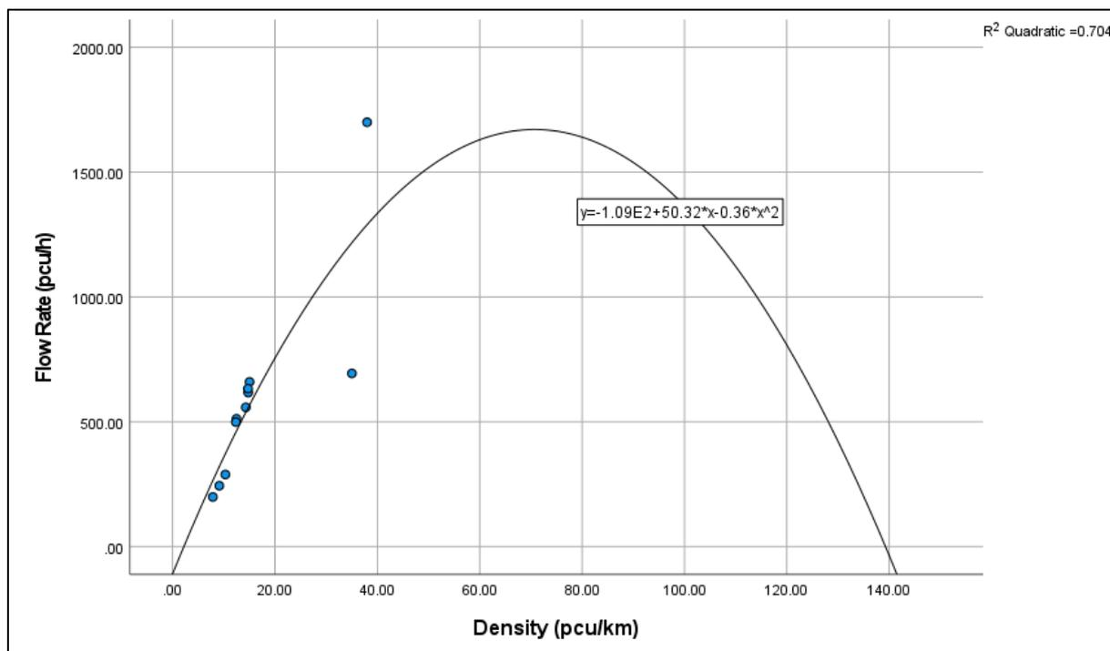
Figure 4.13: Flow-Density Fundamental Diagram for 60 km/h Speed Limit Model.
