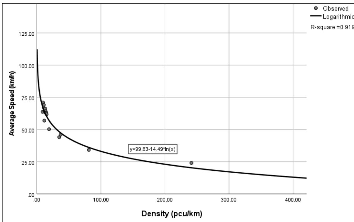
Figure 4.4: Speed-Density Fundamental Diagram for Collector/Distributor Road Model.
