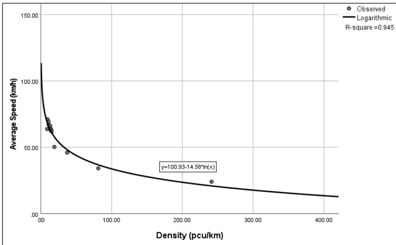
Figure 4.8: Speed-Density Fundamental Diagram for Dual Carriageway Model.
