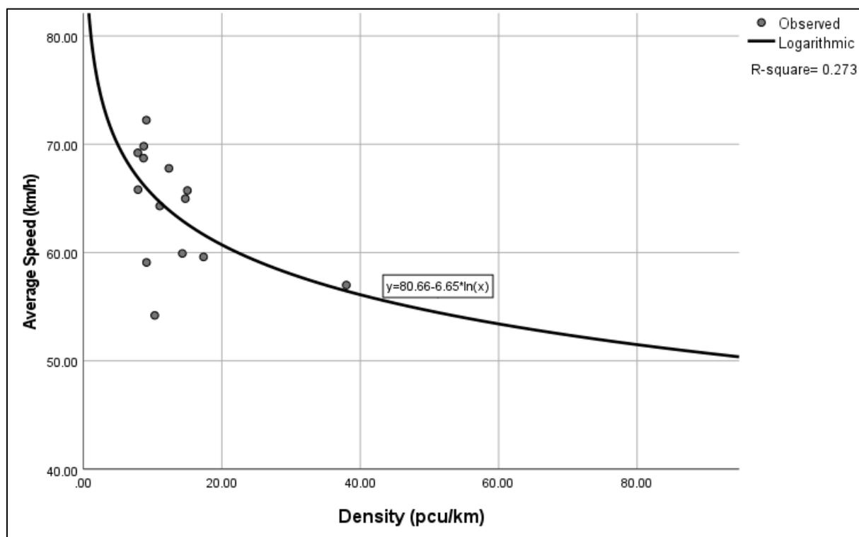
Figure 4.6: Speed-Density Fundamental Diagram for Local Road Model.
