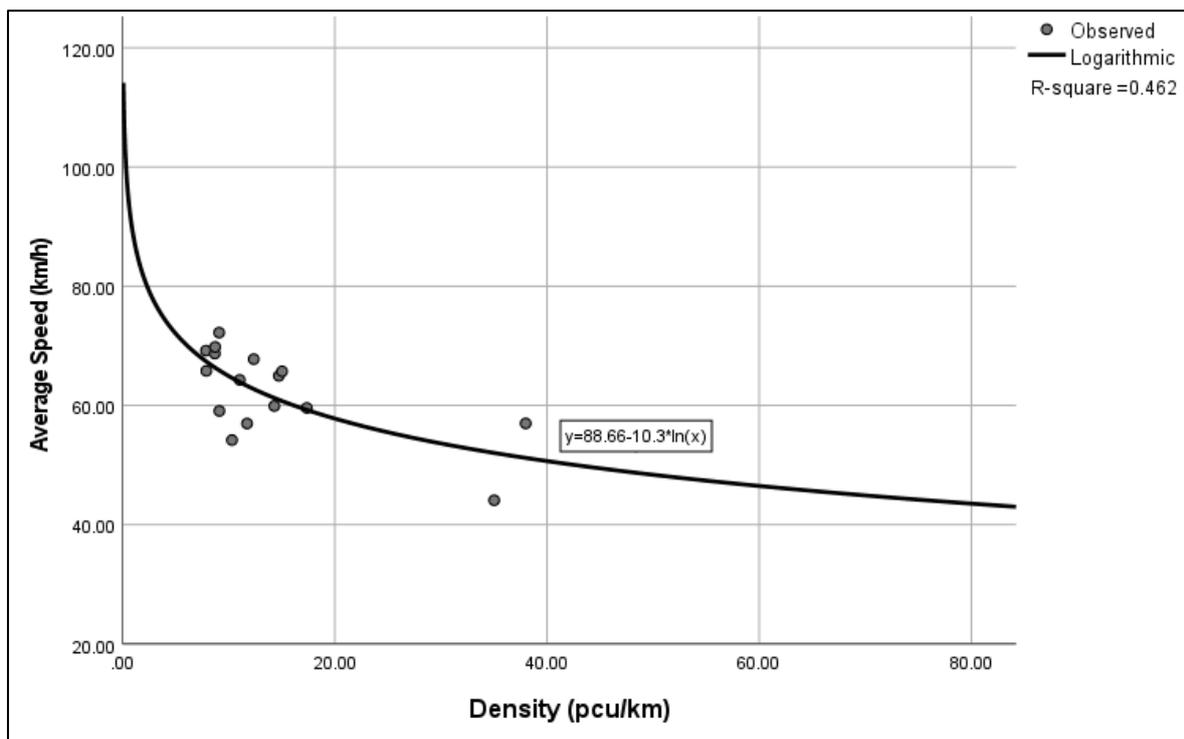
Figure 4.10: Speed-Density Fundamental Diagram for Single Carriageway Model.
