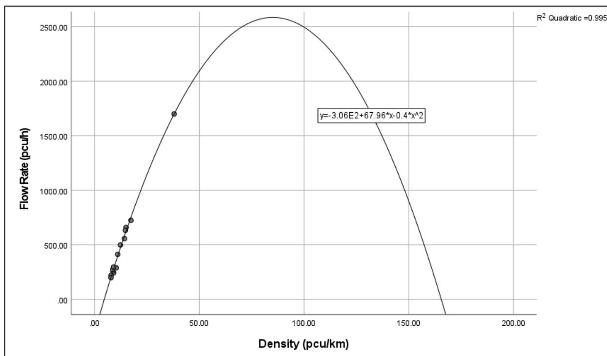
Figure 4.5: Flow-Density Fundamental Diagram for Local Road.
