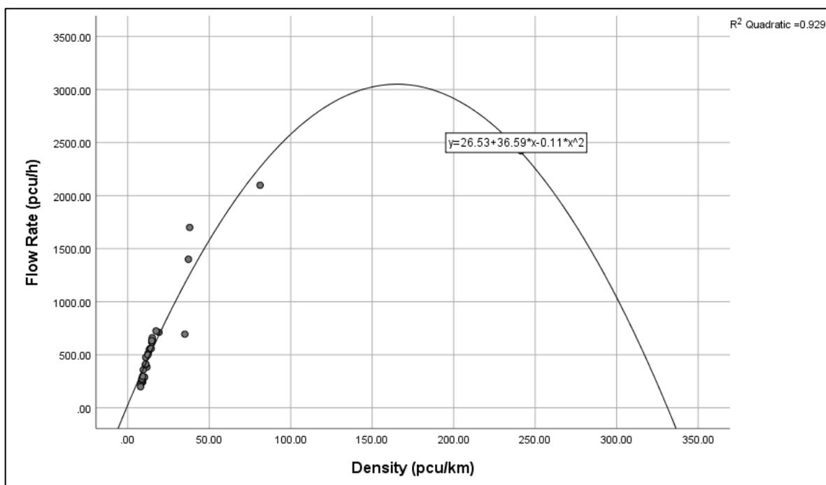
Figure 4.1: Flow-Density Fundamental Diagram for Main Model.
