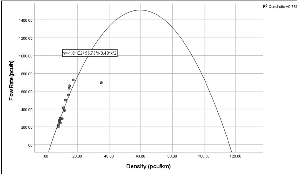
Figure 4.9: Flow-Density Fundamental Diagram for Single Carriageway Model.
