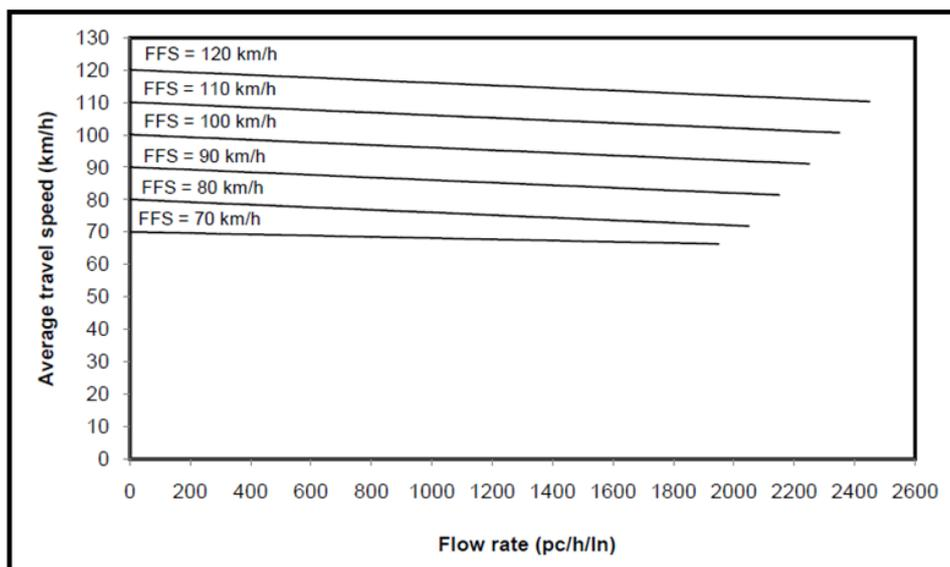
Figure 2.3: Relationship Between Average Travel Speed with Flow Rate for Basic Segment Expressways (Highway Planning Unit Ministry of Works Malaysia, 2011).
