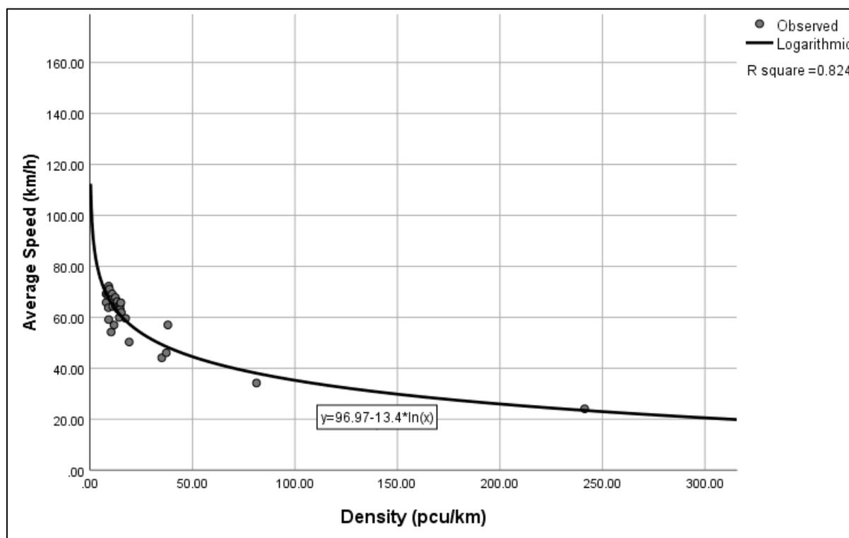
Figure 4.2: Speed-Density Fundamental Diagram for Main Model.
