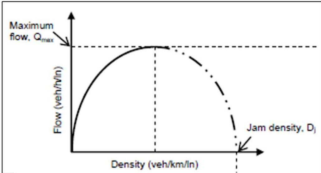
Figure 3.7: Flow-Density Fundamental Diagram (Transportation Research Board, 2016).
