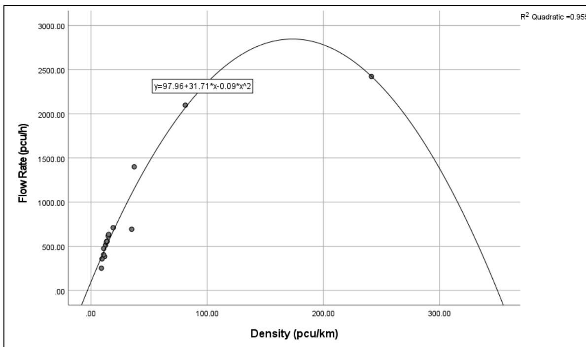
Figure 4.3: Flow-Density Fundamental Diagram for Collector/Distributor Road Model.
