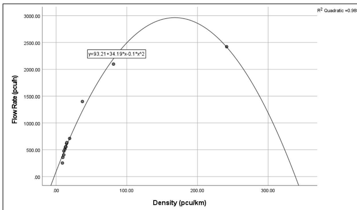
Figure 4.7: Flow-Density Fundamental Diagram for Dual Carriageway Model.
