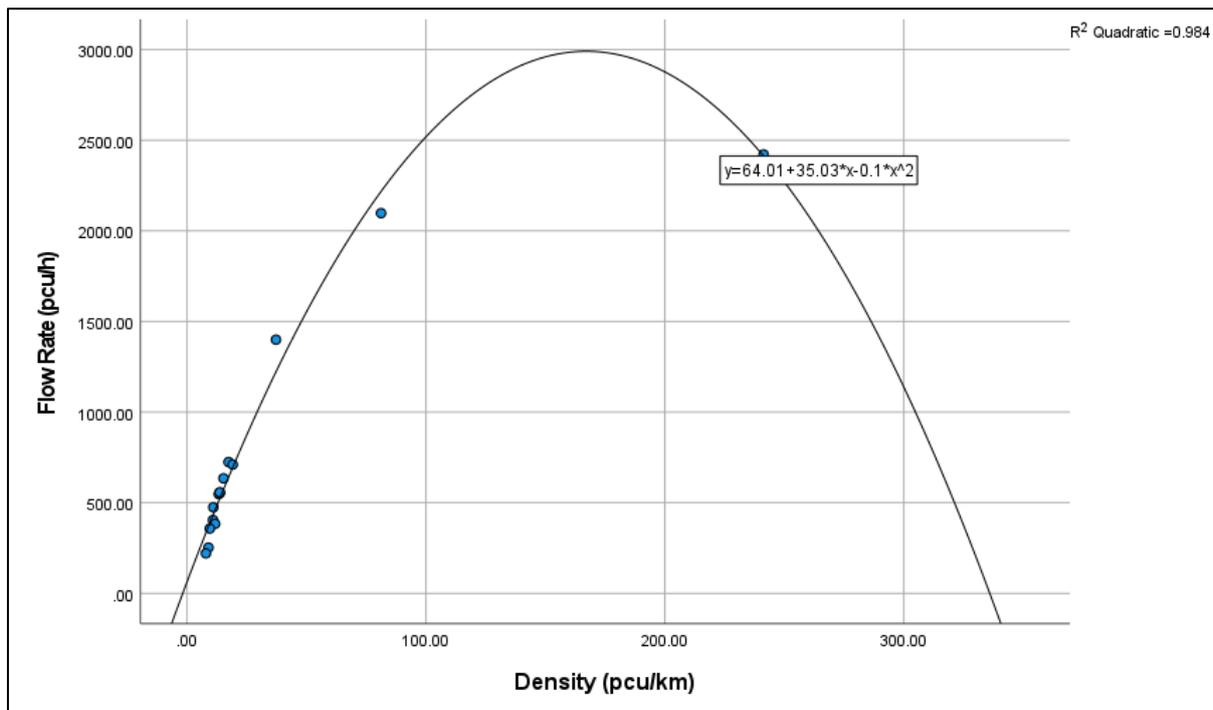
Figure 4.14: Flow-Density Fundamental Diagram for 70 km/h Speed Limit Model.
