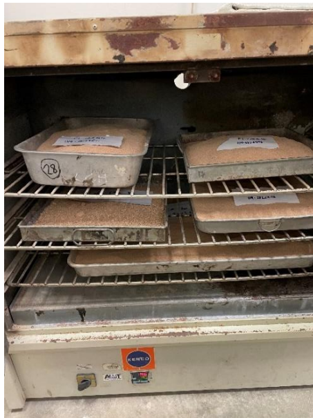
Figure 3.5: The Sand Was Oven-Dried in Oven for 24 Hours.
