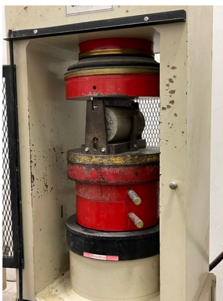
Figure 3.33: Concrete Compression Machine for Splitting Tensile Strength Test Was Set Up.
