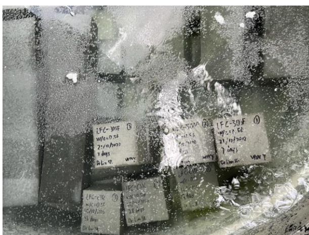
Figure 3.27: Curing Foamed Concrete Specimens in Water Tank.
