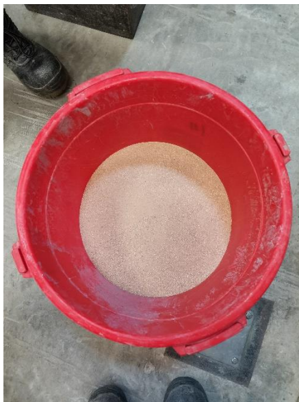
Figure 3.8: The Retained Sieved Fine Aggregate Was Stored in Air-Tight Container.
