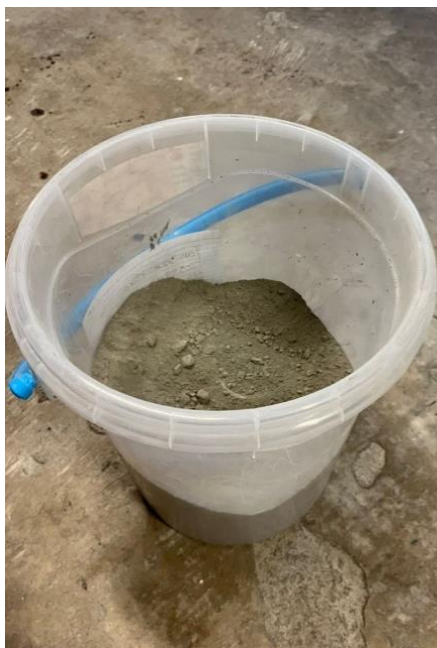
Figure 3.3: Sieved Cement Stored in Air-Tight Container.
