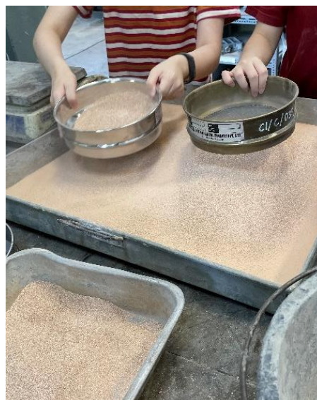
Figure 3.7: The Oven Dried Sand Was Sieved Through a 600 \mu\text{m} Sieve.
