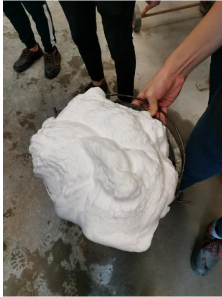
Figure 3.22: Stable Foam Was Used for Production of Foamed Concrete.
