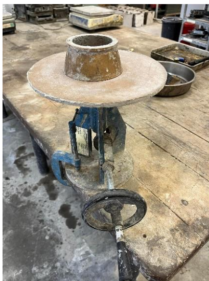
Figure 3.29: The Mould Positioned in the Middle of Flow Table.
