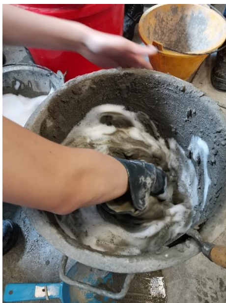
Figure 3.24: Generated Stable Foamed Concrete Was Added and Mixed in Concrete Mix.
