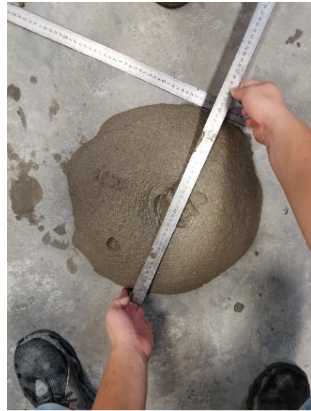
Figure 3.31: Measurement of Slump Spread Diameter.
