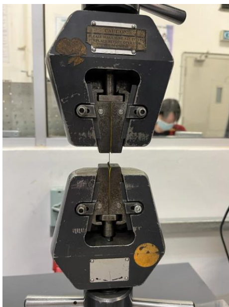
Figure 3.14: Steel Fiber Gripped To Grip Head.
