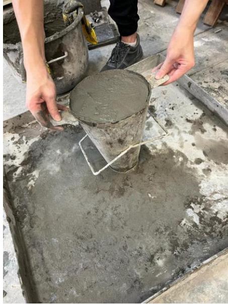
Figure 3.30: The Inverted Slump Cone Was Fully Filled With LFC.
