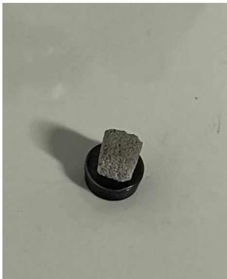
Figure 3.35: Concrete Specimen Mounted on the Pin Stubs.
