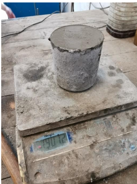
Figure 3.28: Determination of Density of Foamed Concrete at Fresh State.
