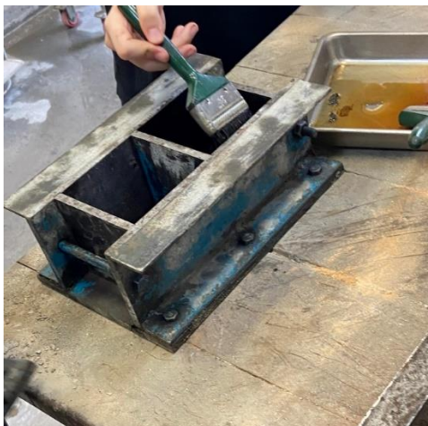
Figure 3.19: The Surface of Cubic Mould Was Applied with Oil.
