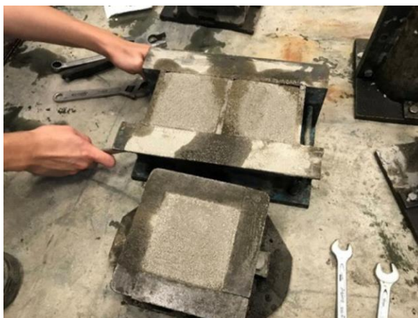
Figure 3.26: Specimens Demould Process.
