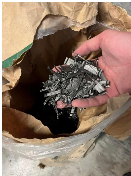
Figure 3.12: Hooked-End Type Steel Fiber.
