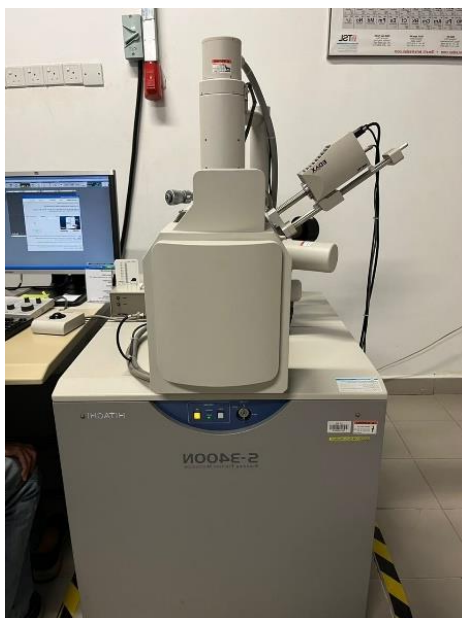
Figure 3.37: Hitachi S-3600N SEM.
