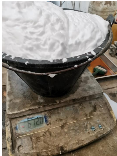
Figure 3.23: The Weight of Generated Foam Was Taken Before Added Into the Concrete Mix.
