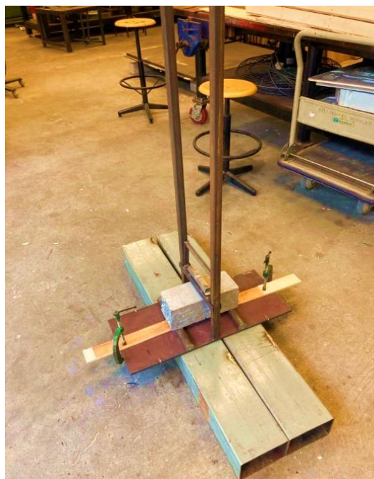
Figure 3.32: Repeated Drop Weight Impact Test.
