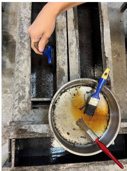
Figure 3.19: A Thin Layer of Oil Was Coated on the Mould's Surface.
