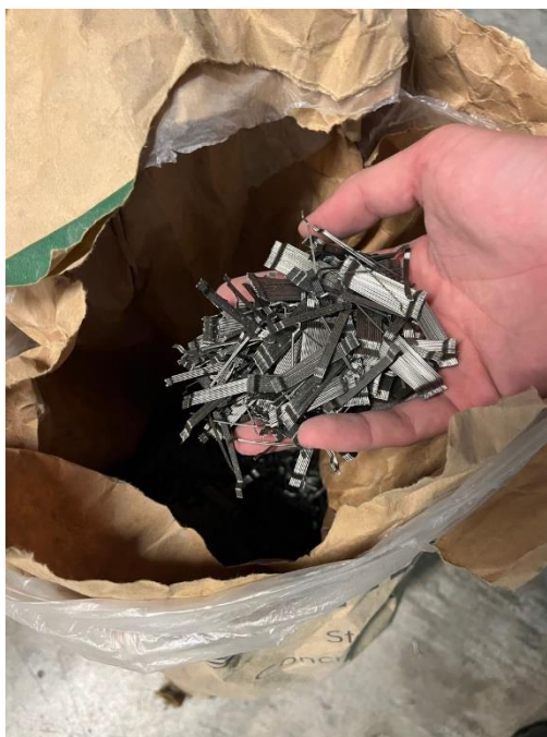
Figure 3.13: Stahlcon Hooked-End Steel Fiber HE 0.55/35.
