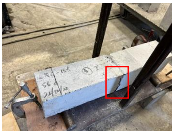
Figure 5.12: Fracture Pattern of LRC-15 % SF.
