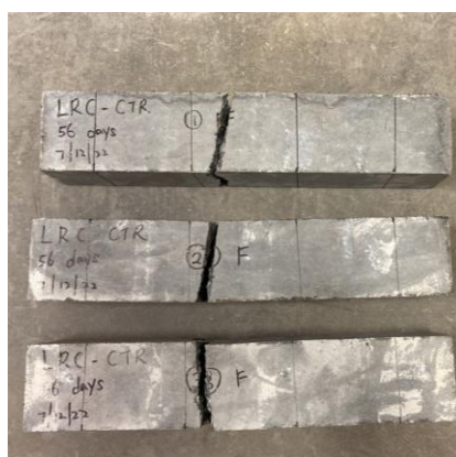
Figure 5.8: Flexural Failure of LRC-CTR.
