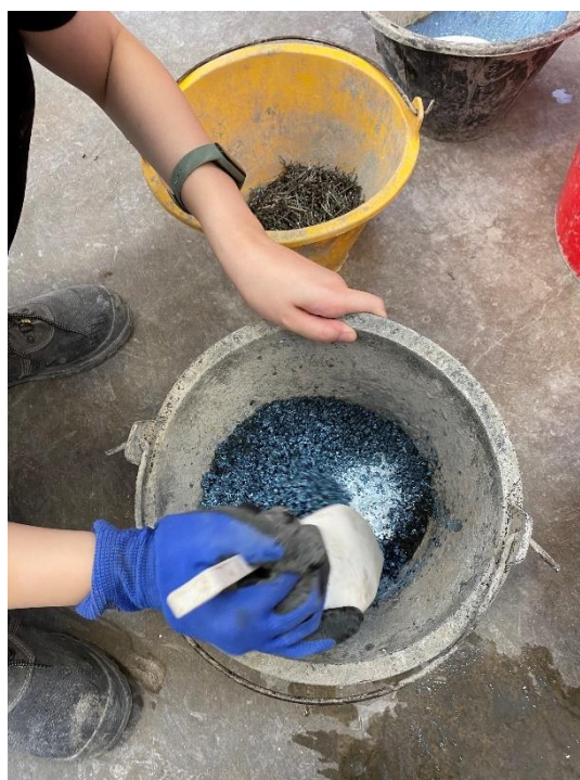
Figure 3.21: Crumb Rubber Coated With SBR Latex.
