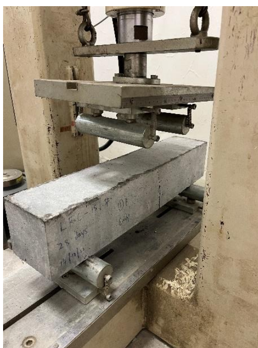
Figure 3.31: Flexural Strength Test.
