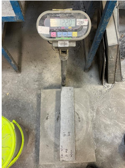
Figure 3.28: Concrete Was Weighted Using Weighing Machine.
