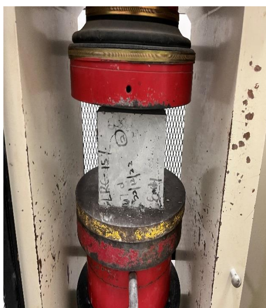
Figure 3.29: Compressive Strength Test.
