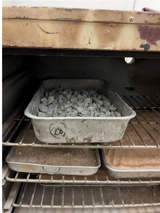
Figure 3.6: Coarse and Fine Aggregate Oven-Dried in the Oven.
