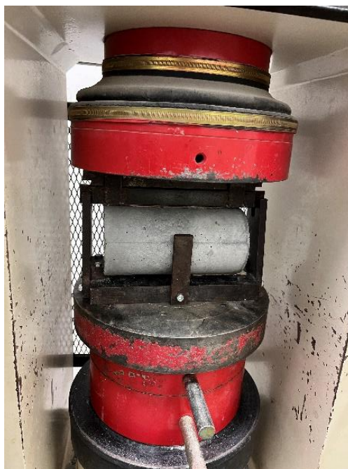
Figure 3.30: Splitting Tensile Strength Test.
