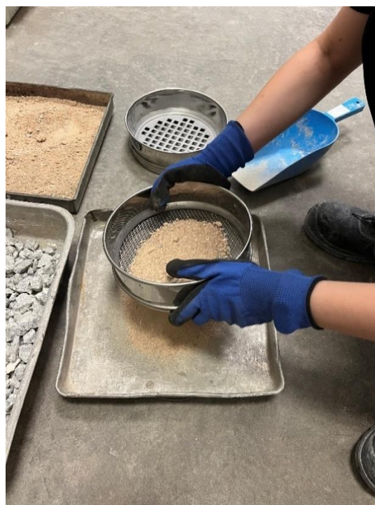
Figure 3.5: Fine Aggregates Retained on the Receiving Pan.
