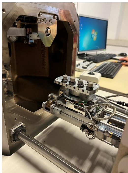
Figure 3.34: Specimens Were Placed in Vacuum Chamber.
