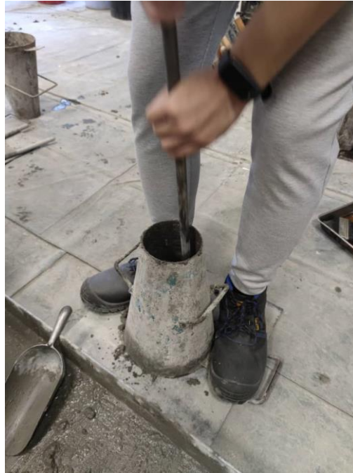
Figure 3.22: Concrete Mix Was Consolidated Using Tamping Rod.
