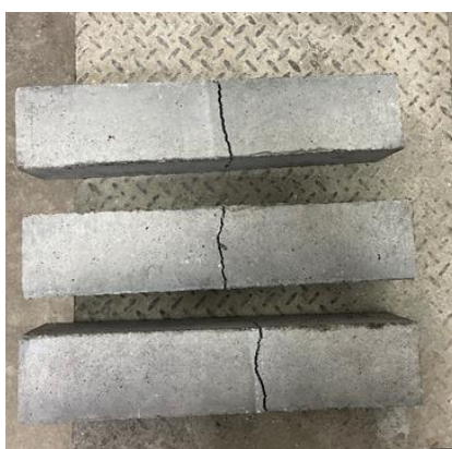
Figure 5.9: Flexural Failure of LRC-15 % SF.
