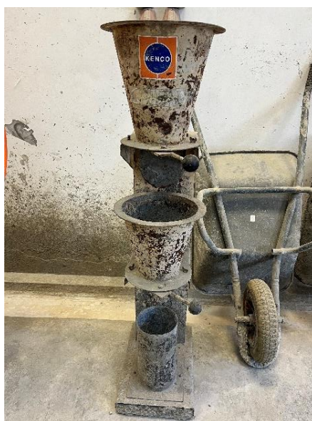
Figure 3.24: Compacting Factor Test.
