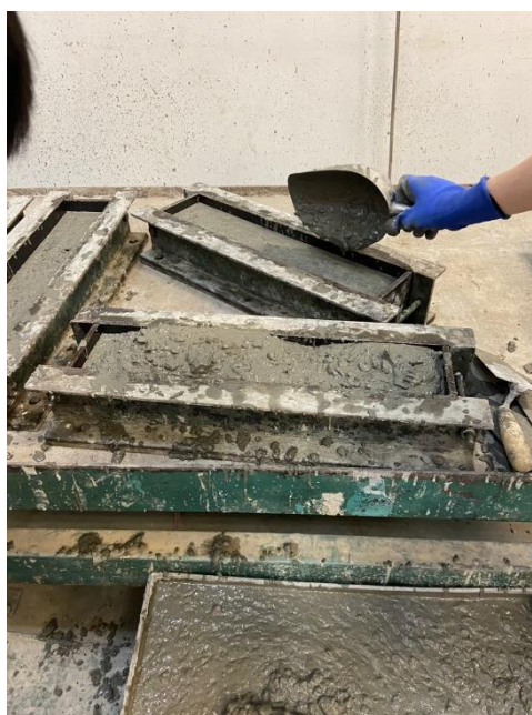
Figure 3.25: Fresh Concrete Was Transferred to the Prism Mould.
