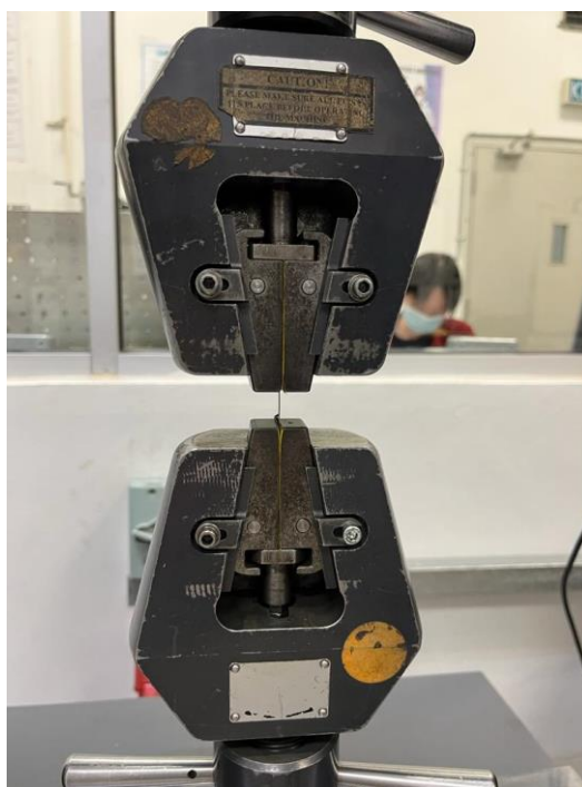
Figure 3.14: Preparation of Tensile Test.
