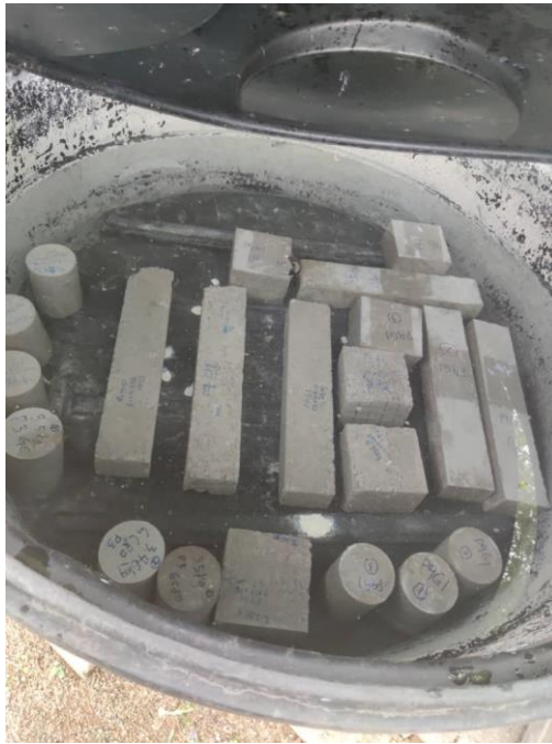
Figure 3.26: Water Curing for the Concrete Specimens.
