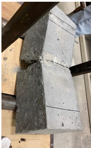
Figure 5.13: Fracture Pattern of LRC-CTR (200 mm).
