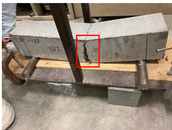
Figure 5.11: Fracture Pattern of LRC-CTR.
