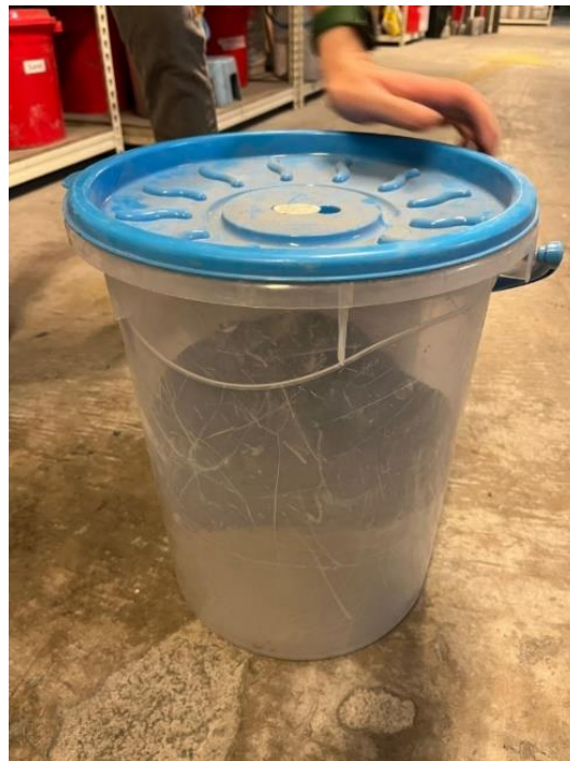
Figure 3.4: Sieved OPC in an Air-Tight Container.
