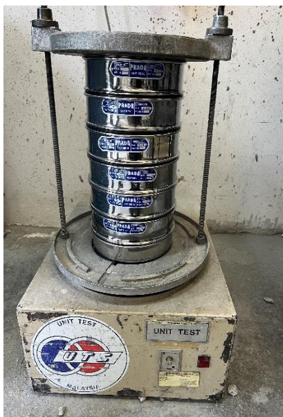
Figure 3.8: Set Up of Sieve Analysis Test.
