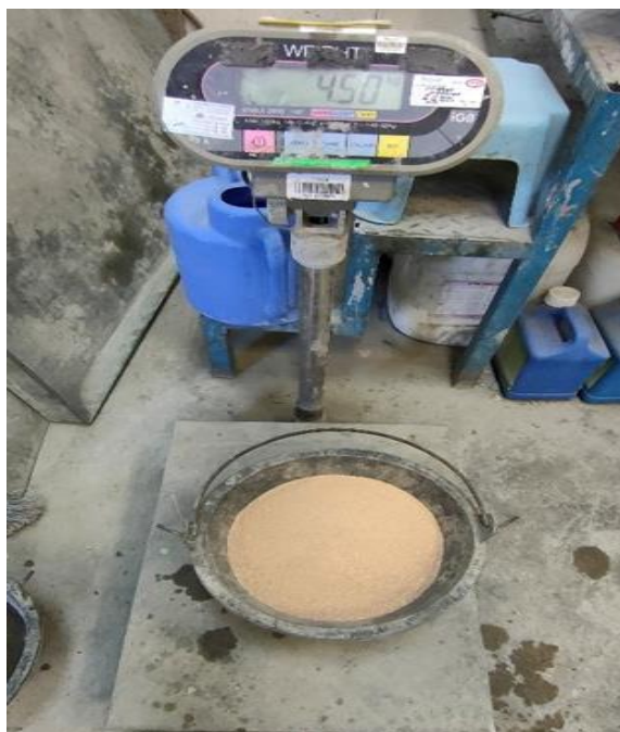
Figure 3.20: Fine Aggregate Was Weighted.
