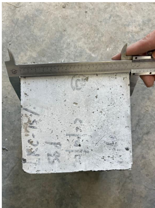
Figure 3.27: Dimension Was Measured Using Vernier Calliper.
