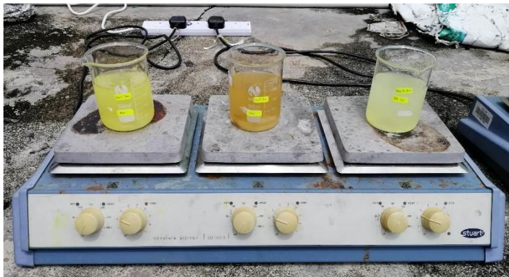
Figure 3.6: Experimental Setup for Photoreduction of Cr(VI).
