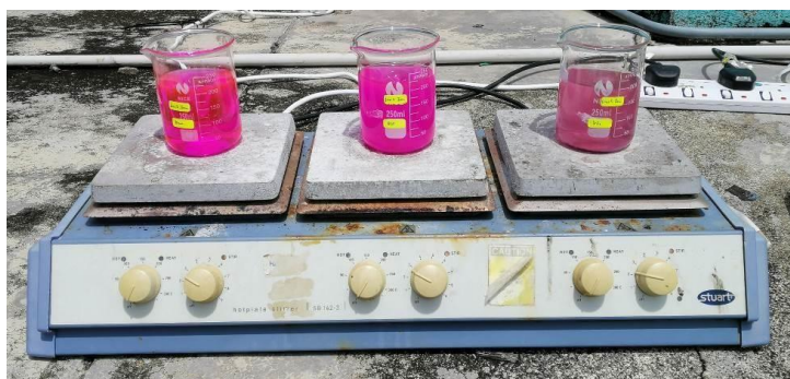
Figure 3.5: Experimental Setup for Photodegradation of Rhodamine B.
