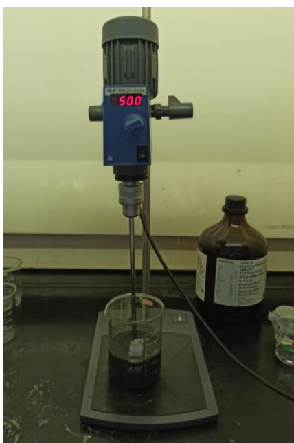
Figure 3.4: Compounding blending by using IKA RW 20 Digital
