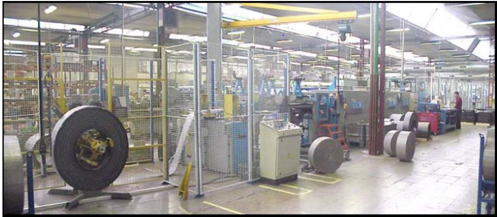
Figure 2.8 Process line of gasket calendaring and stamping ( Description of production processes, 2012 )
