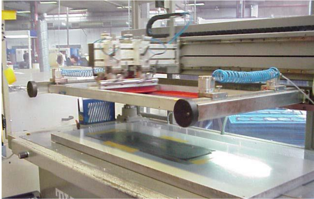
Figure 2.10: Gasket is under silk-screen printing ( Description of production processes, 2012 )
