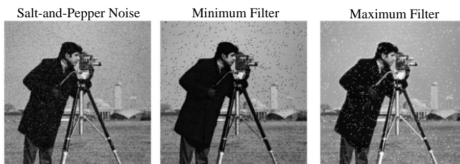
Figure 2.11: Denoising Outputs Using Minimum and Maximum Filters.
