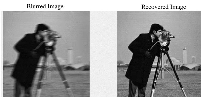
Figure 2.18: Example of Output from Wiener Filter Deconvolution.
