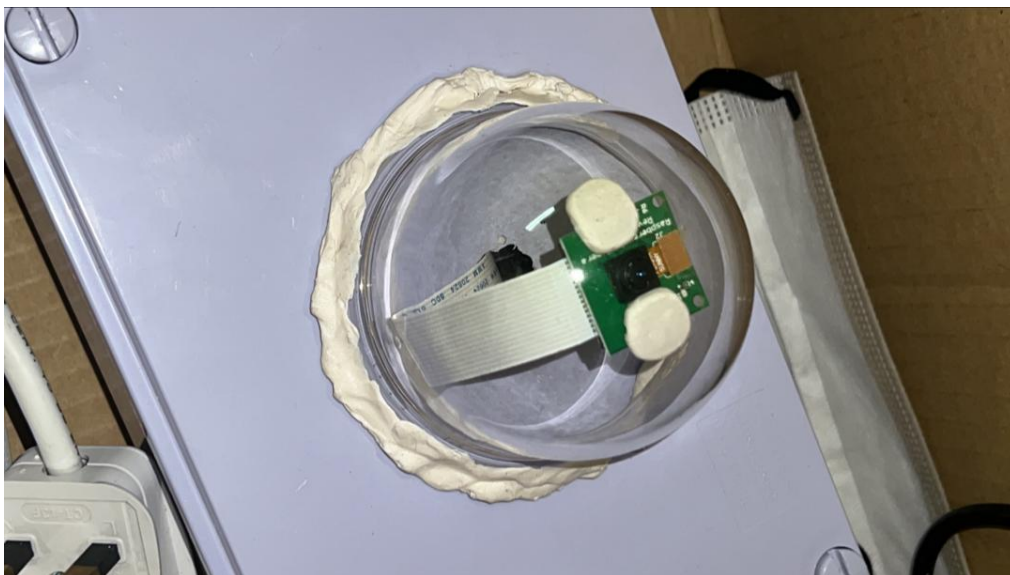
Figure 4.6: Position of Raspberry Pi Camera when moved to the tip of the dome
