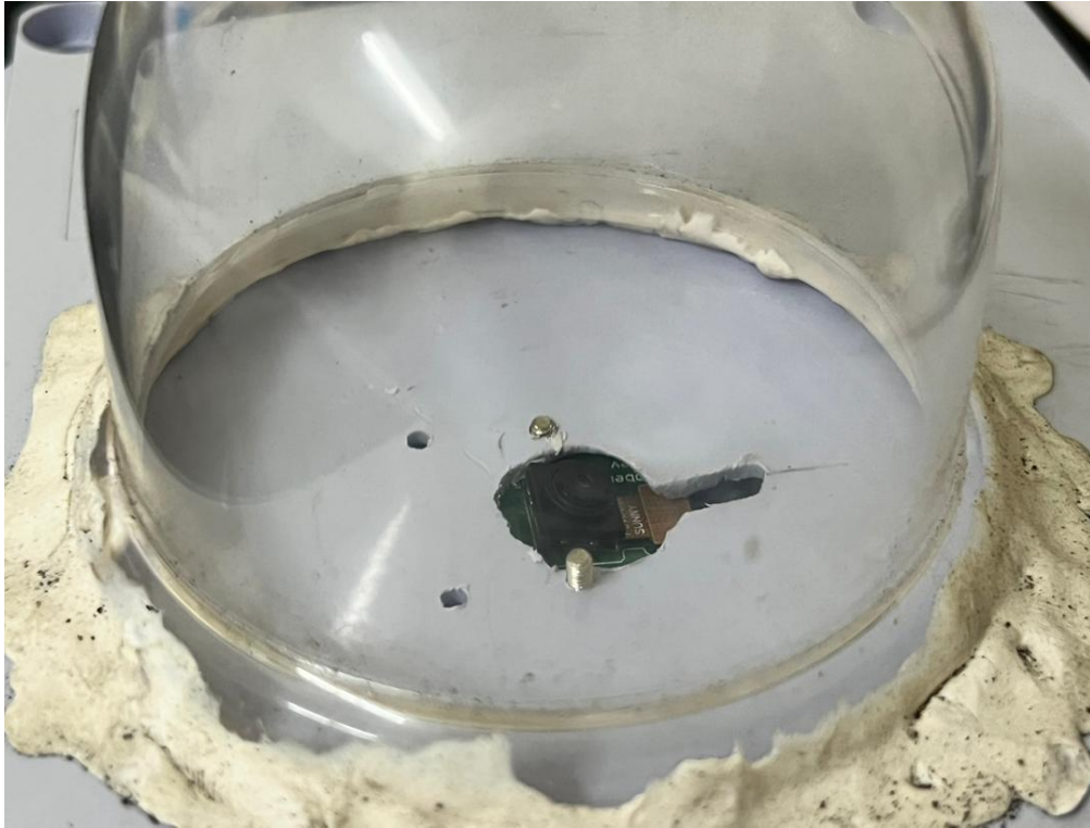
Figure 4.5: Initial position of the Raspberry Pi Camera ( beneath the waterproof casing)
