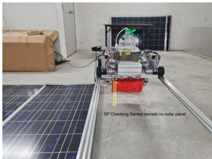
Figure 4.37: SP Checking Sensor senses the absence of solar panel.
