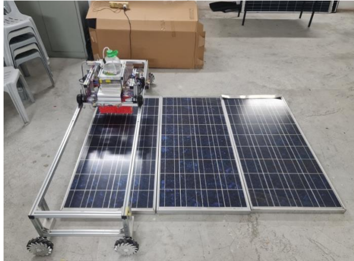
Figure 4.35: Robot positioned at the first cleaning column.
