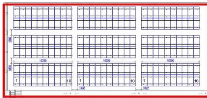
Figure 3.1: Nine Arrays of Solar Panels on Industrial Rooftop.
