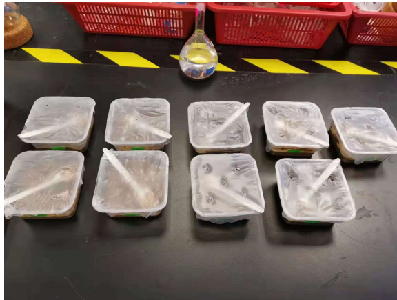
Figure 3.18: Treated soil samples that were incubated in plastic container with covered for 30 days
