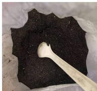
Figure 3.4: Rice husk-derived biochar
