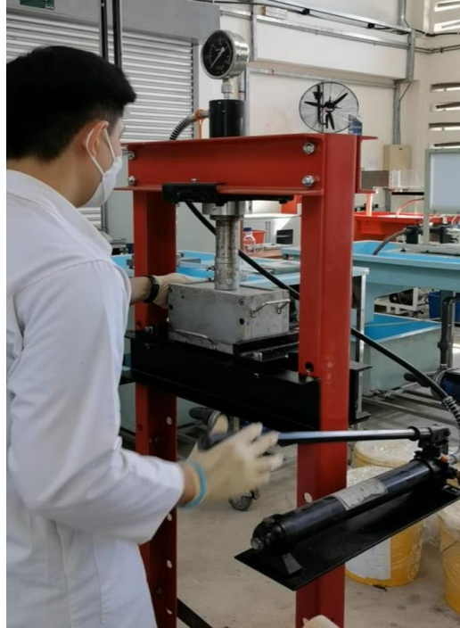
Figure 3.8: Compression of the CSB Specimen by 20 Tons Hydraulic Shop Press.
