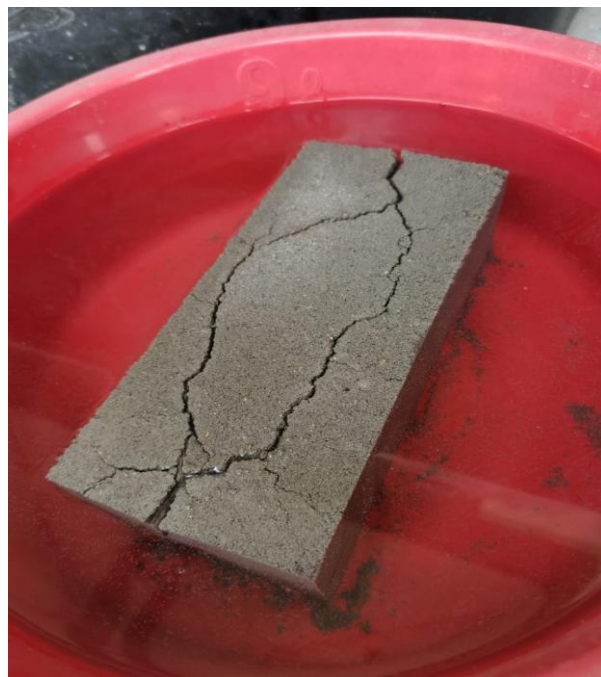
Figure 4.2: The Immersed CSB Specimen Substituted with Untreated AD in Water on Day 3.
