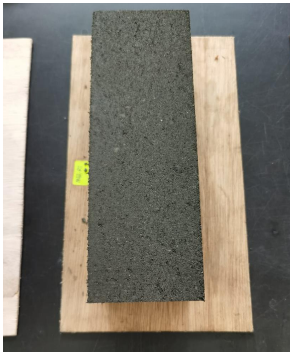
Figure 3.9: Demoulding of the CSB specimen.
