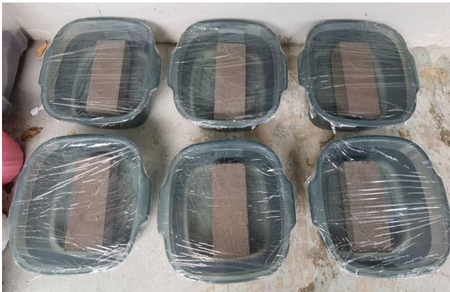
Figure 3.20: Leaching of Metal Ions from The Specimens.
