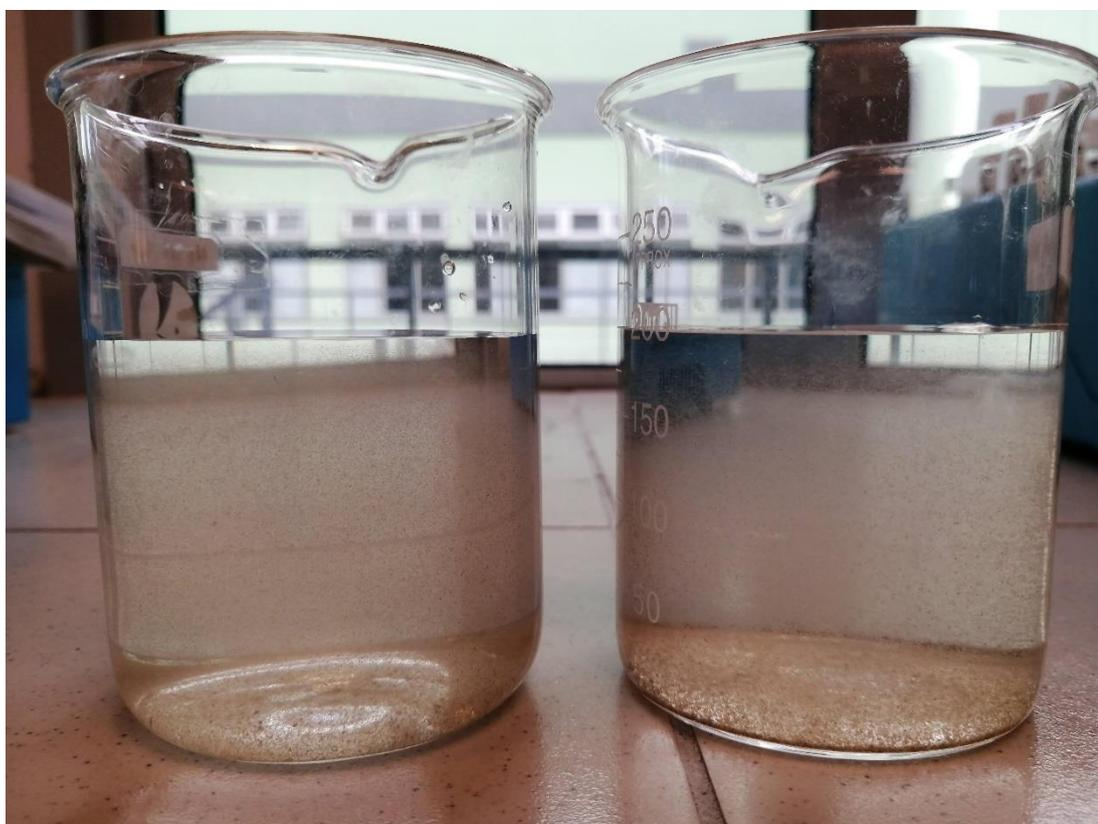
**Figure 4.4: Denser sludge in the effluent collected from copper CW-MFC (left) compared to iron CW-MFC (right)**
