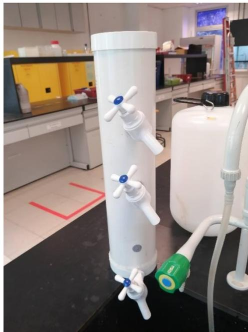
**Figure 3.4: Setup for anaerobic pre-treatment of AS**
