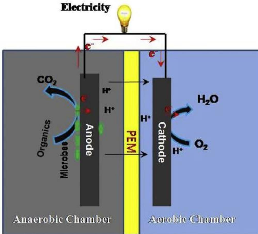
Figure 2.2: A typical setup of MFC (Srivastava et al., 2019)
