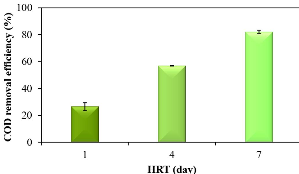
**Figure 4.5: Effect of HRT on the removal of COD in copper CW-MFC under closed circuit connection**
