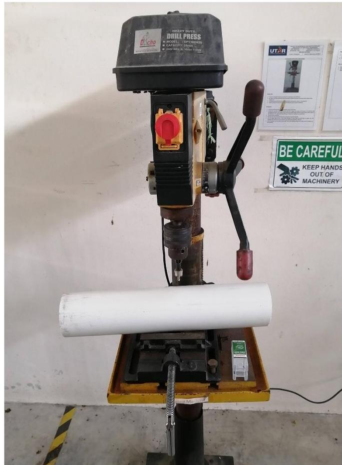
**Figure A3: Drilling holes through PVC pipe by using drill press**
