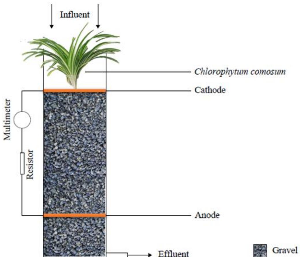
Figure 3.2: Schematic diagram of CW-MFC
