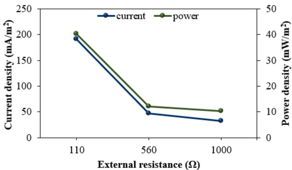
Figure 4.8: Effect of external resistances on generation current and power density
