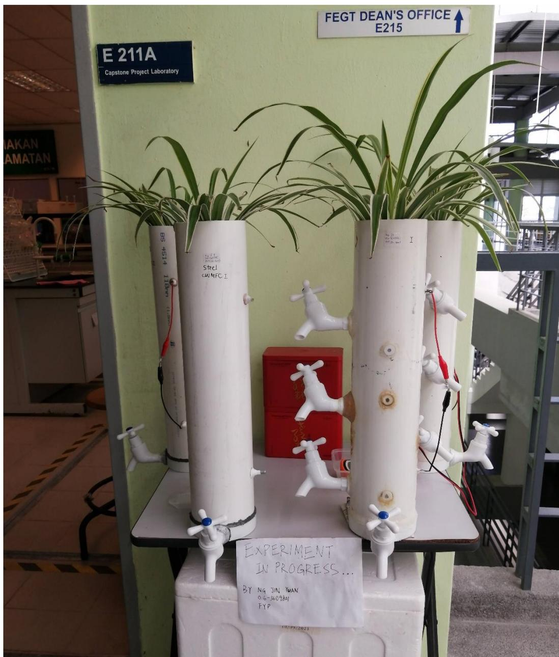
**Figure A9: Completed setup of copper and iron CW-MFCs under different circuit connections**
