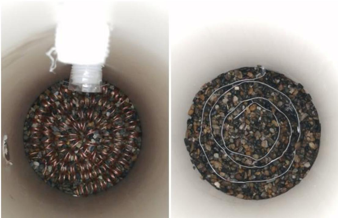
**Figure A6: Placement of copper (left) and iron (right) anodes in the respective CW-MFC systems**
