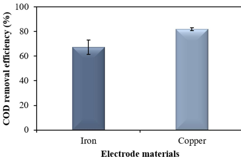
**Figure 4.3: Effect of electrode material on the COD removal efficiency by close circuit CW-MFC**
