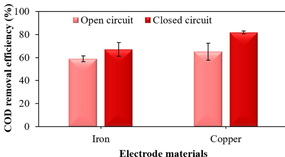
**Figure 4.2: COD removal efficiency of copper CW-MFC and iron CW-MFC under closed circuit and open circuit connections**
