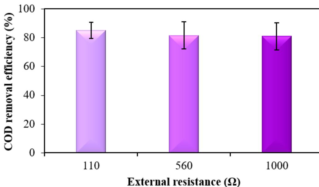
**Figure 4.6: Effect of external resistance on the removal of COD in copper CW-MFC under closed circuit connection**
