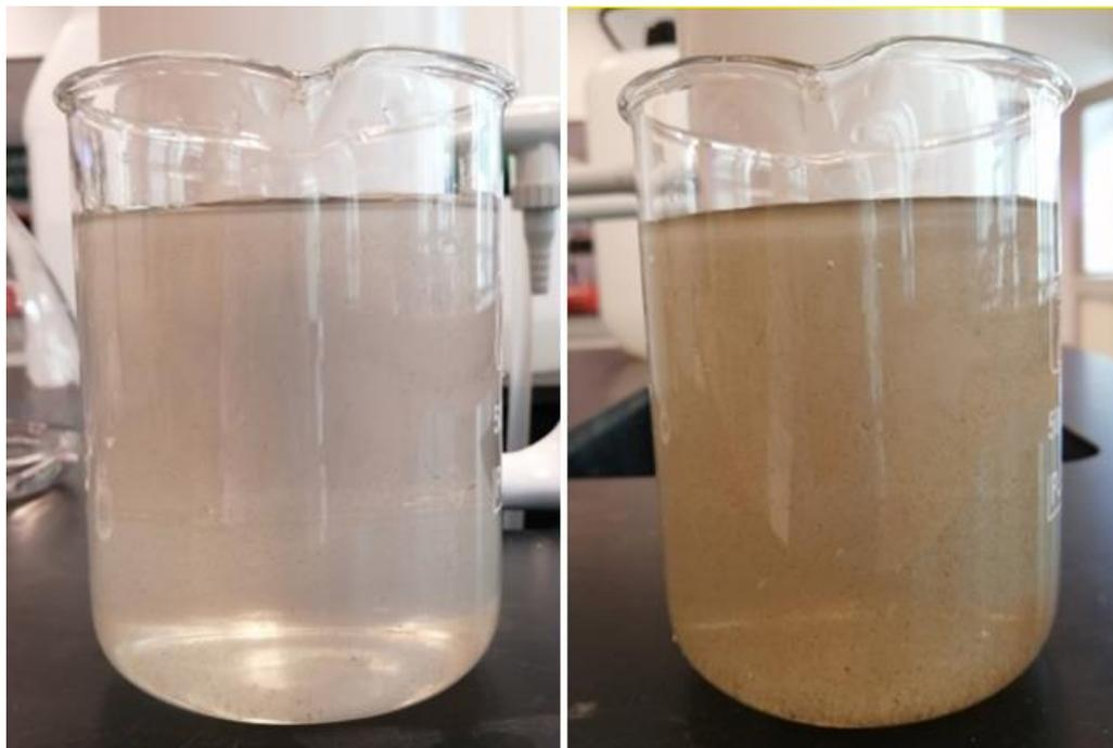
**Figure A4: Activated sludge before (left) and after (right) anaerobic pre-treatment**
