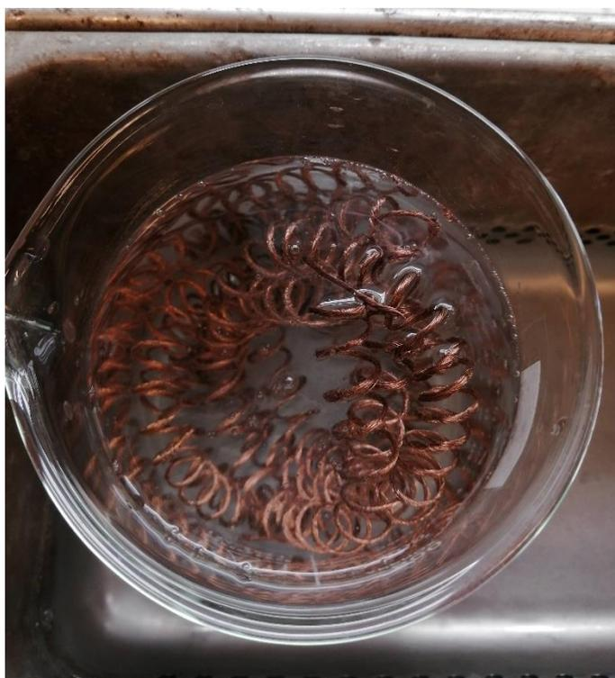
**Figure A5: Removing impurities on electrode surface**
