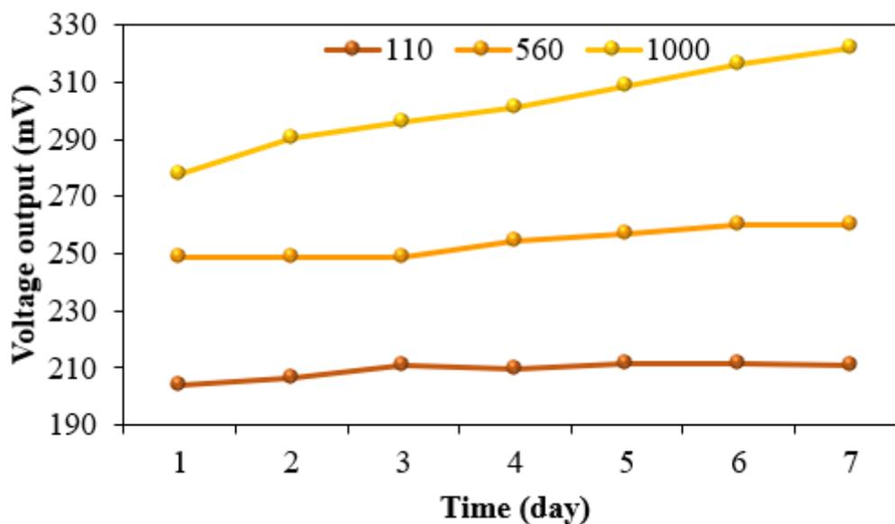
Figure 4.7: Effect of external resistance on voltage output
