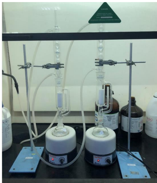
Figure 3.11: Apparatus set-up for Soxhlet Extraction.
