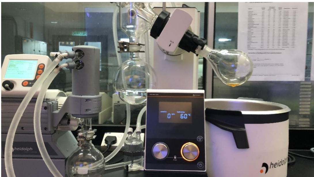
Figure 3.13: Rotary evaporator is used for the removal of n-hexane from crude lipid.
